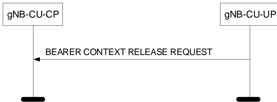
Figure 8.3.5.2-1: Bearer Context Release Request procedure: Successful Operation.
