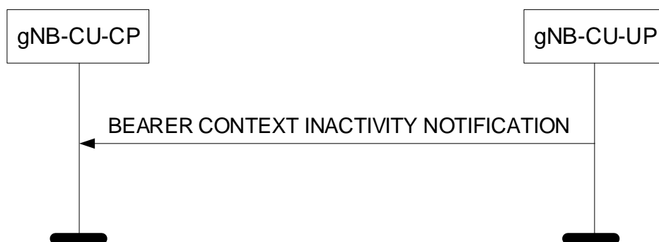
Figure 8.3.6.2-1: Bearer Context Inactivity Notification procedure: Successful Operation.
