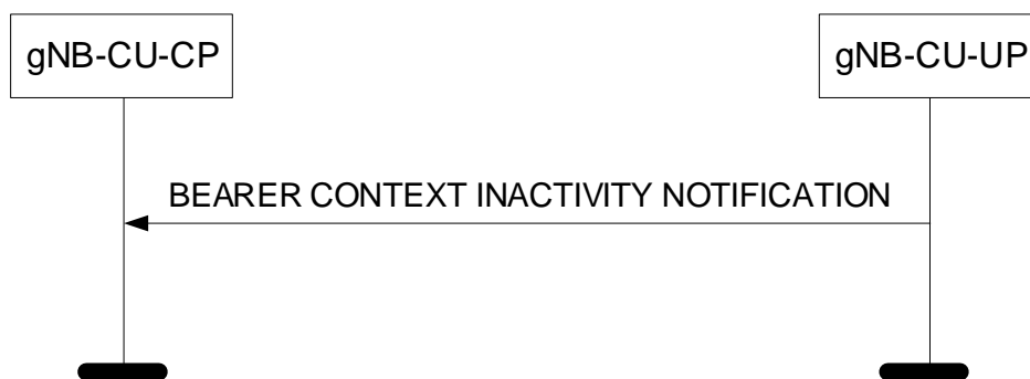
Figure 8.3.6.2-1: Bearer Context Inactivity Notification procedure: Successful Operation.
