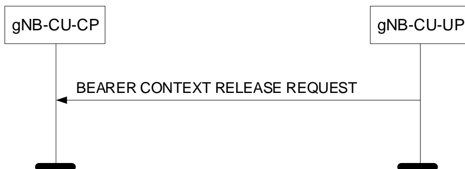
Figure 8.3.5.2-1: Bearer Context Release Request procedure: Successful Operation.
