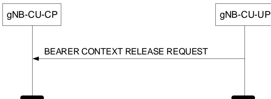
Figure 8.3.5.2-1: Bearer Context Release Request procedure: Successful Operation.
