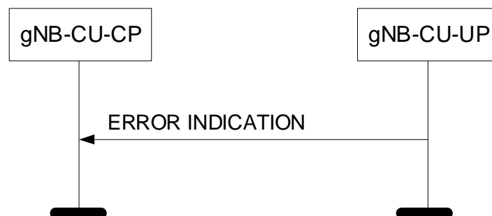
Figure 8.2.2.2-2: Error Indication procedure, gNB-CU-UP originated. Successful operation.
