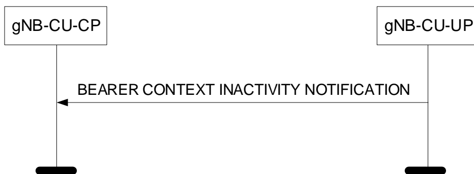
Figure 8.3.6.2-1: Bearer Context Inactivity Notification procedure: Successful Operation.
