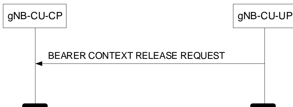
Figure 8.3.5.2-1: Bearer Context Release Request procedure: Successful Operation.
