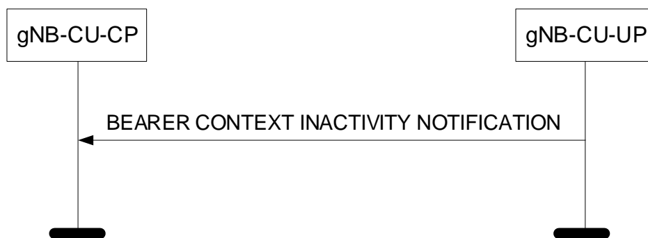
Figure 8.3.6.2-1: Bearer Context Inactivity Notification procedure: Successful Operation.
