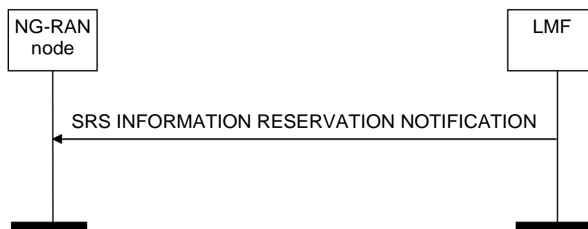
Figure 8.2.14.2-1: SRS Information Reservation Notification procedure, successful operation
