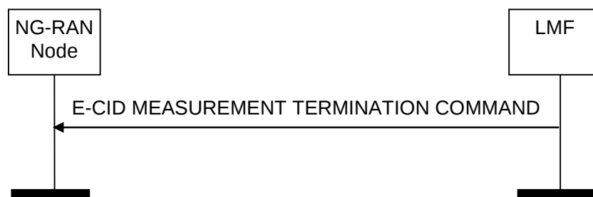
Figure 8.2.4.2-1: E-CID Measurement Termination procedure, successful operation
