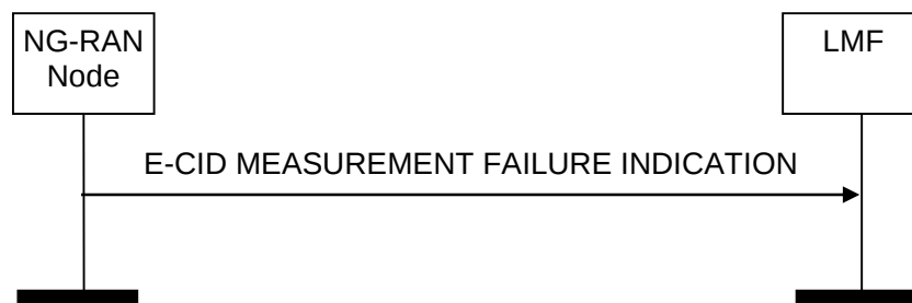
Figure 8.2.2.2-1: E-CID Measurement Failure Indication, successful operation
