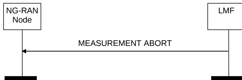
Figure 8.5.4.2.1: Measurement Abort Procedure: Successful Operation.
