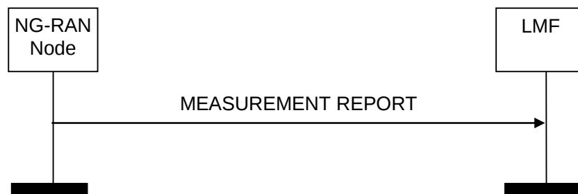
Figure 8.5.2.2.1: Measurement Report procedure. Successful operation.
