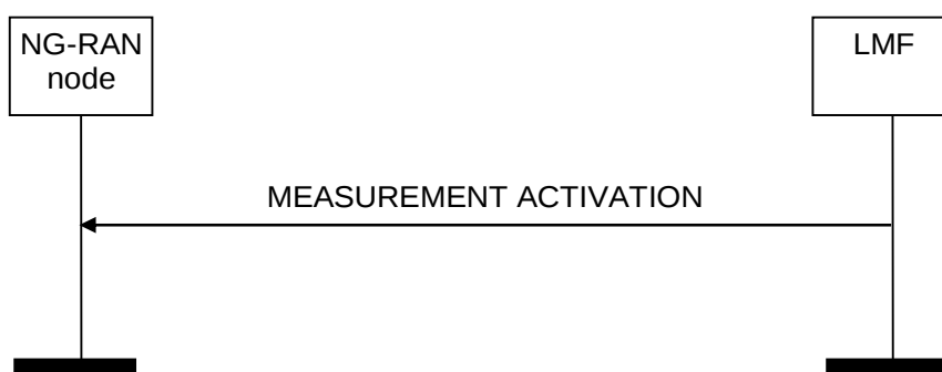
Figure 8.2.13.2-1: Measurement Activation procedure, successful operation
