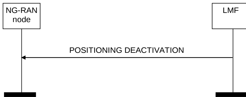
Figure 8.2.10.2-1: Positioning Deactivation procedure, successful operation
