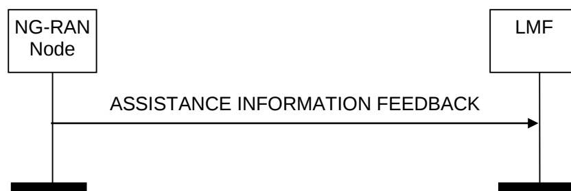
Figure 8.4.2.2-1: Assistance Information Feedback procedure
