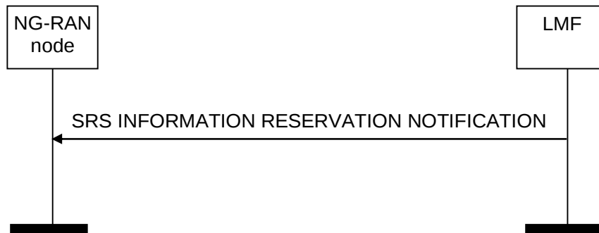
Figure 8.2.14.2-1: SRS Information Reservation Notification procedure, successful operation
