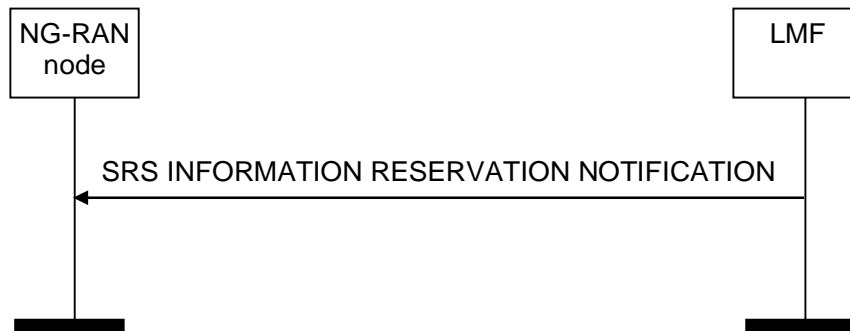
Figure 8.2.14.2-1: SRS Information Reservation Notification procedure, successful operation
