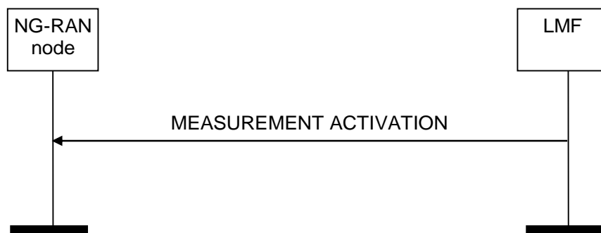
Figure 8.2.13.2-1: Measurement Activation procedure, successful operation
