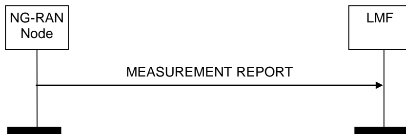
Figure 8.z.2.2.1: Measurement Report procedure. Successful operation.
