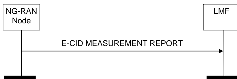
Figure 8.2.3.2-1: E-CID Measurement Report procedure, successful operation
