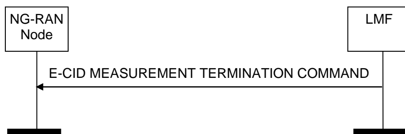
Figure 8.2.4.2-1: E-CID Measurement Termination procedure, successful operation
