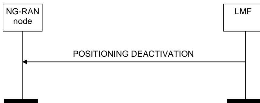
Figure 8.2.10.2-1: Positioning Deactivation procedure, successful operation
