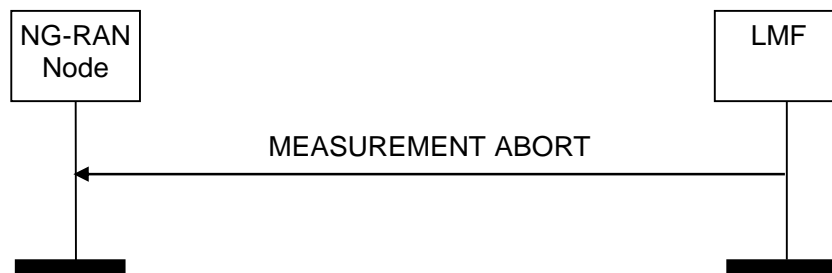
Figure 8.5.4.2.1: Measurement Abort Procedure: Successful Operation.
