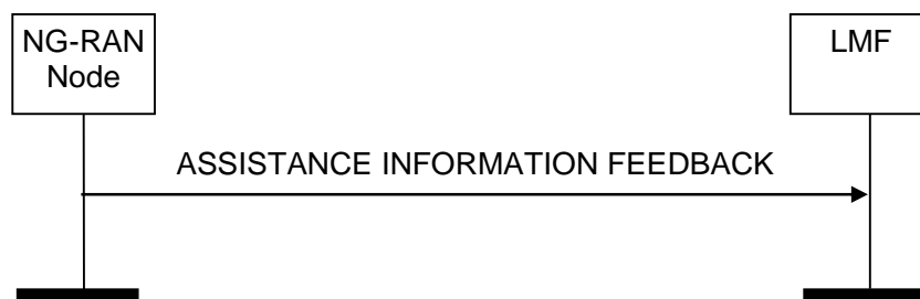
Figure 8.4.2.2-1: Assistance Information Feedback procedure
