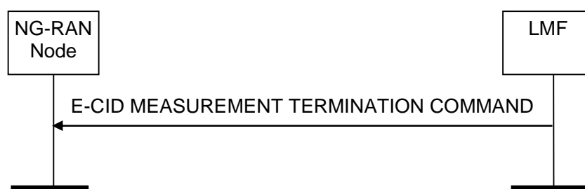
Figure 8.2.4.2-1: E-CID Measurement Termination procedure, successful operation
