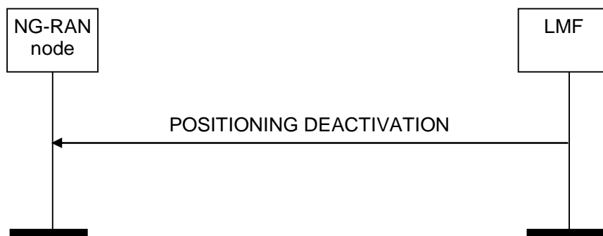
Figure 8.2.10.2-1: Positioning Deactivation procedure, successful operation
