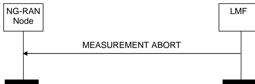
Figure 8.5.4.2.1: Measurement Abort Procedure: Successful Operation.
