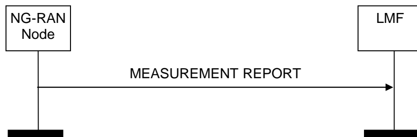
Figure 8.z.2.2.1: Measurement Report procedure. Successful operation.
