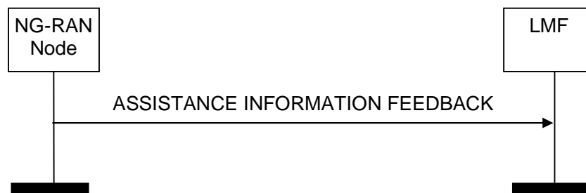
Figure 8.4.2.2-1: Assistance Information Feedback procedure
