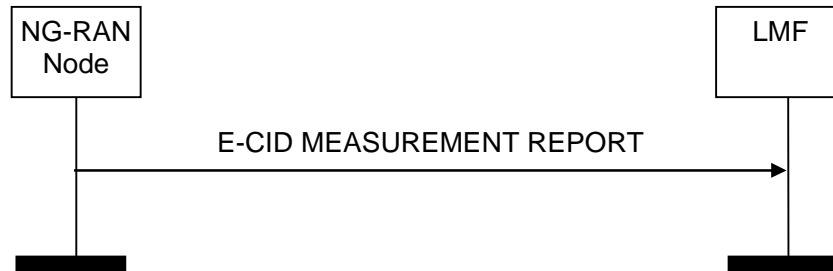
Figure 8.2.3.2-1: E-CID Measurement Report procedure, successful operation
