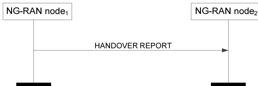
Figure 8.4.8.2-1: Handover Report, successful operation
