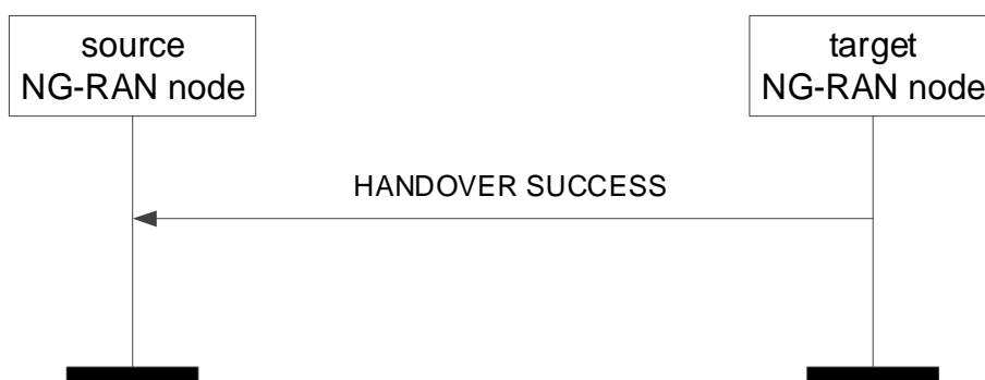
Figure 8.2.8.2-1: Handover Success, successful operation
