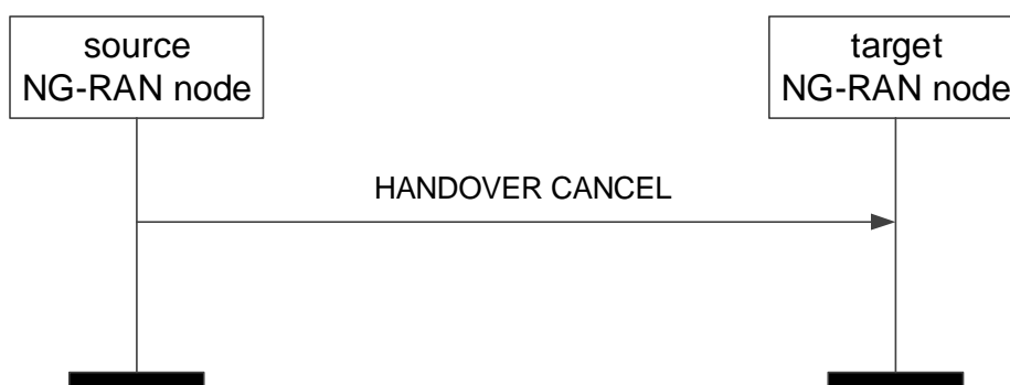
Figure 8.2.3.2-1: Handover Cancel, successful operation
