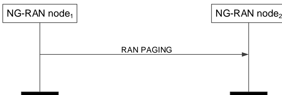
Figure 8.2.5.2-1: RAN Paging: successful operation
