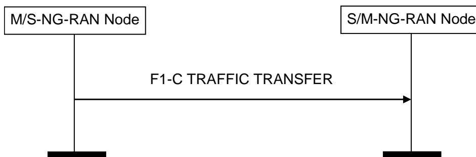
Figure 8.5.1.2-1: F1-C Traffic Transfer procedure, successful operation
