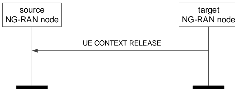
Figure 8.2.7.2-1: UE Context Release, successful operation for handover
