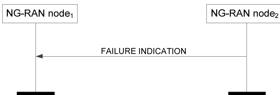
Figure 8.4.7.2-1: Failure Indication, successful operation
