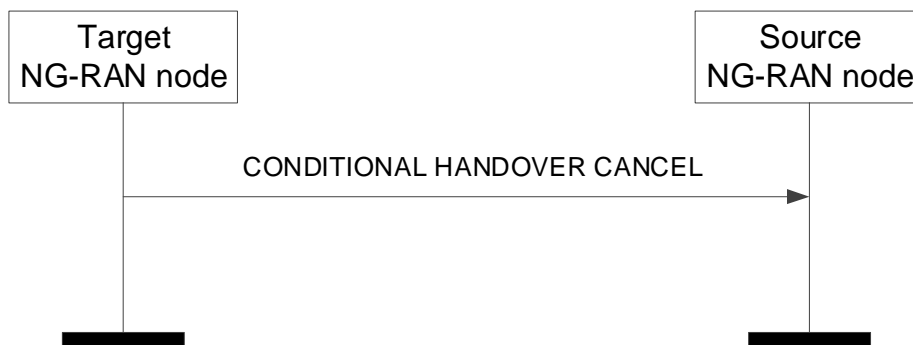
Figure 8.2.9.2-1: Conditional Handover Cancel, successful operation
