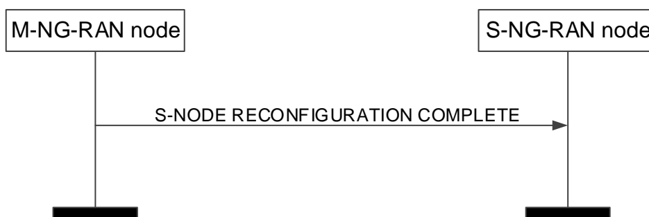
Figure 8.3.2.2-1: S-NG-RAN node Reconfiguration Complete procedure, successful operation.
