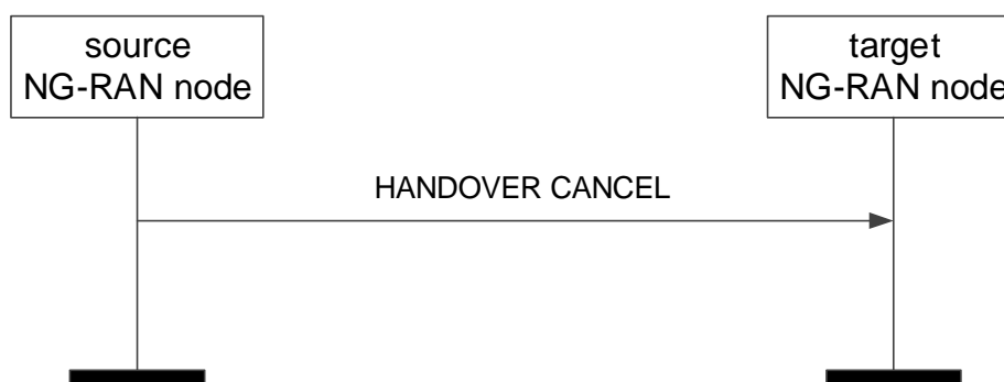
Figure 8.2.3.2-1: Handover Cancel, successful operation
