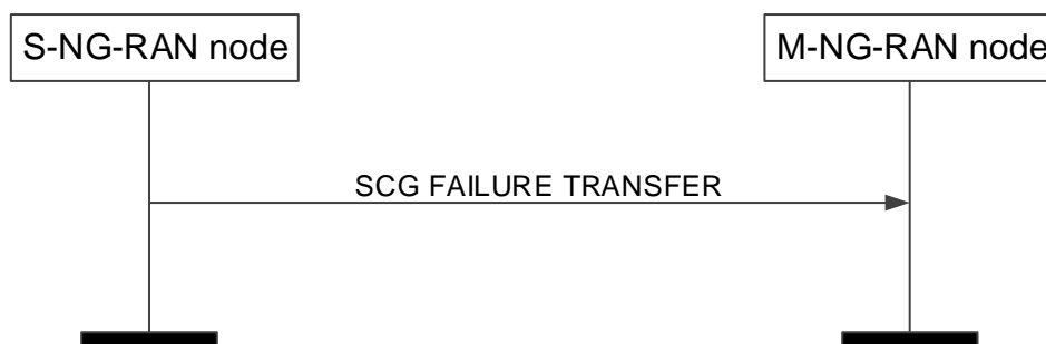
Figure 8.3.18.2-1: SCG Failure Information Transfer, successful operation
