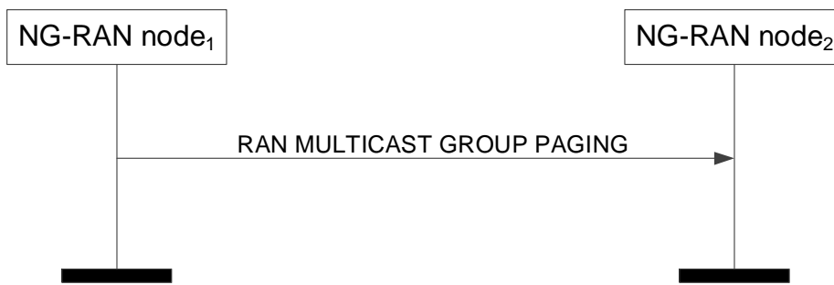
Figure 8.2.11.2-1: RAN Multicast Group Paging, successful operation
