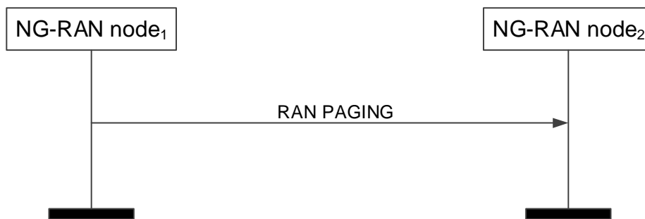
Figure 8.2.5.2-1: RAN Paging: successful operation
