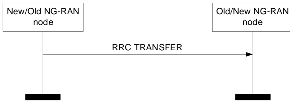
Figure 8.3.9.2-2: RRC Transfer procedure for SDT, successful operation.
