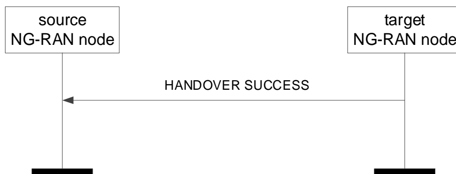
Figure 8.2.8.2-1: Handover Success, successful operation
