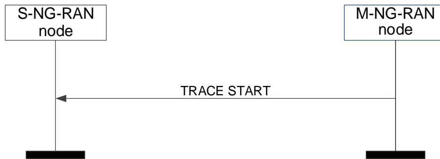
Figure 8.3.14.2-1: Trace Start, successful operation
