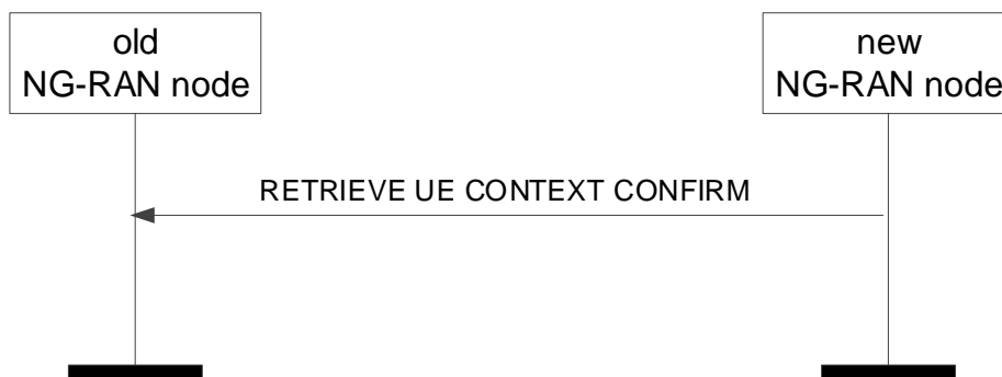
Figure 8.2.12.2-1: Retrieve UE Context Confirm, successful operation
