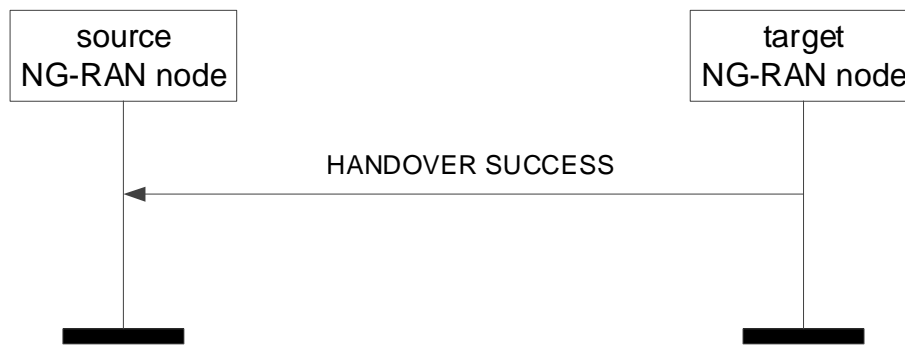
Figure 8.2.8.2-1: Handover Success, successful operation
