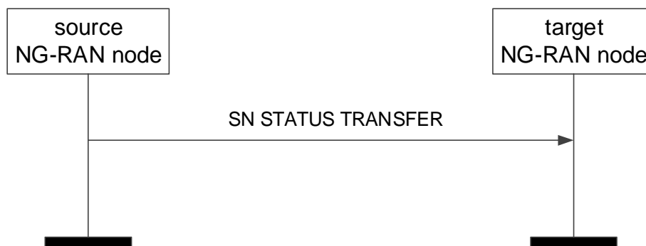
Figure 8.2.2.2-1: SN Status Transfer, successful operation
