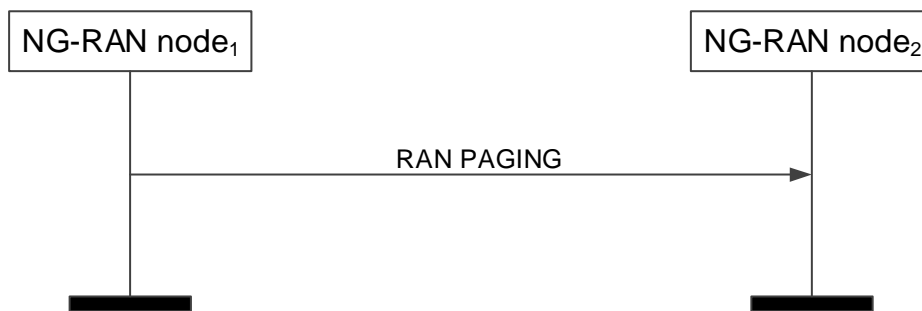
Figure 8.2.5.2-1: RAN Paging: successful operation
