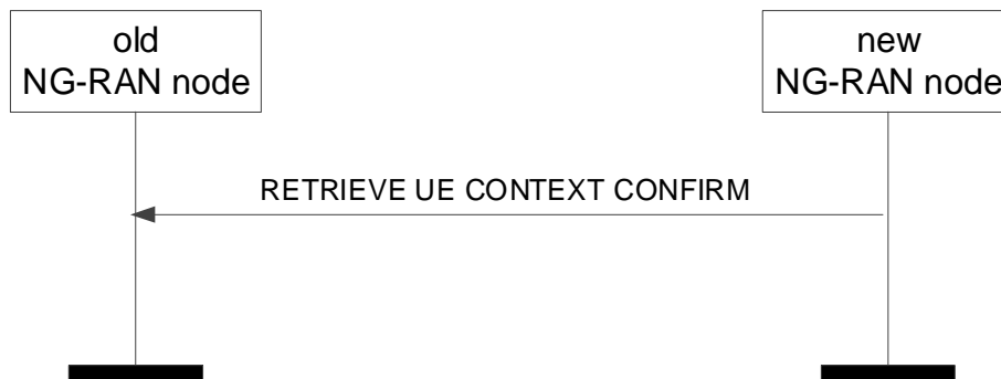
Figure 8.2.12.2-1: Retrieve UE Context Confirm, successful operation
