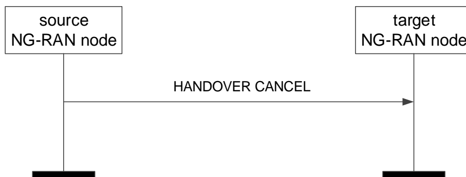
Figure 8.2.3.2-1: Handover Cancel, successful operation
