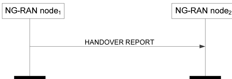
Figure 8.4.8.2-1: Handover Report, successful operation
