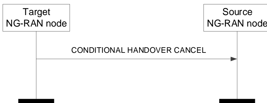
Figure 8.2.9.2-1: Conditional Handover Cancel, successful operation
