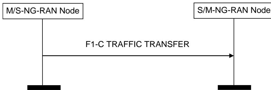
Figure 8.5.1.2-1: F1-C Traffic Transfer procedure, successful operation
