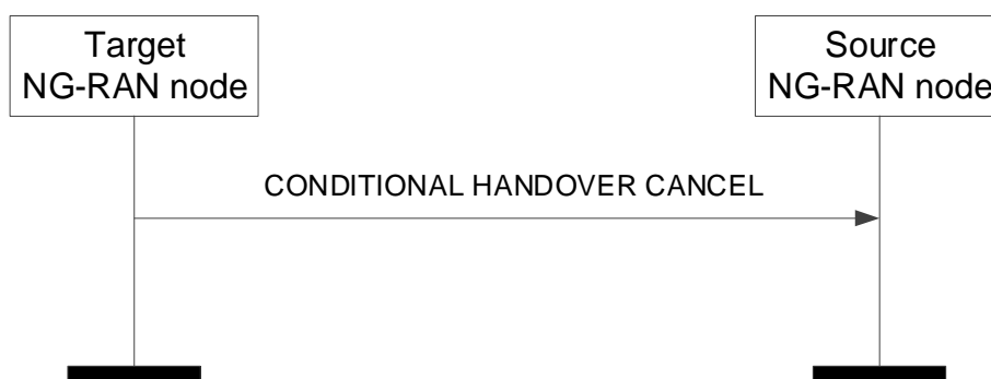
Figure 8.2.9.2-1: Conditional Handover Cancel, successful operation
