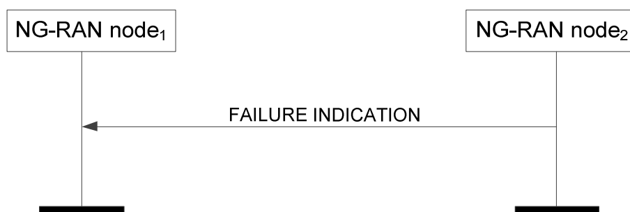
Figure 8.4.7.2-1: Failure Indication, successful operation
