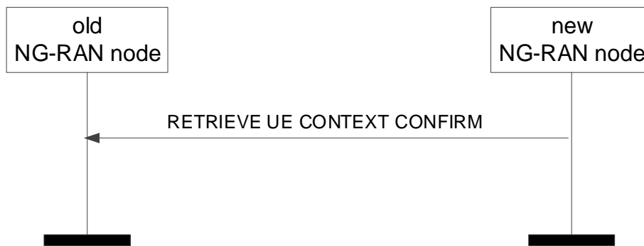
Figure 8.2.12.2-1: Retrieve UE Context Confirm, successful operation
