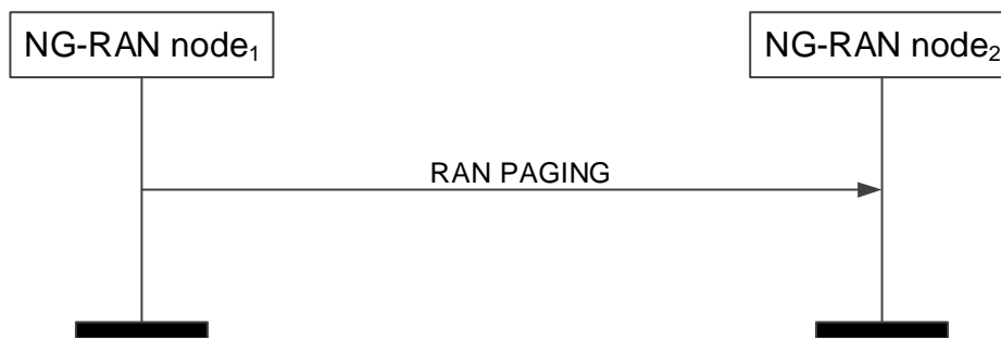
Figure 8.2.5.2-1: RAN Paging: successful operation
