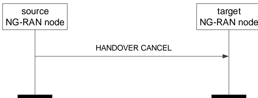
Figure 8.2.3.2-1: Handover Cancel, successful operation
