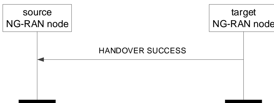
Figure 8.2.8.2-1: Handover Success, successful operation
