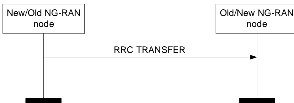
Figure 8.3.9.2-2: RRC Transfer procedure for SDT, successful operation.
