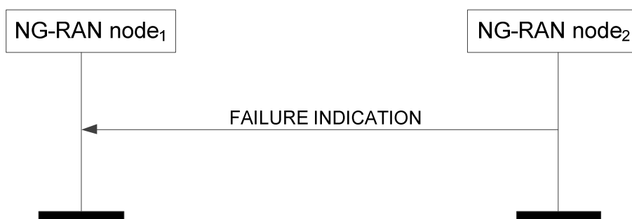
Figure 8.4.7.2-1: Failure Indication, successful operation
