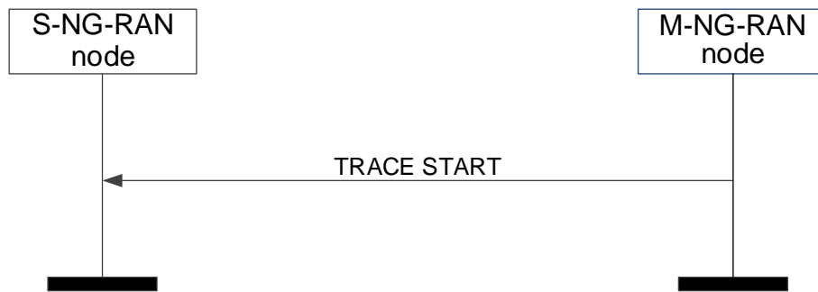
Figure 8.3.14.2-1: Trace Start, successful operation
