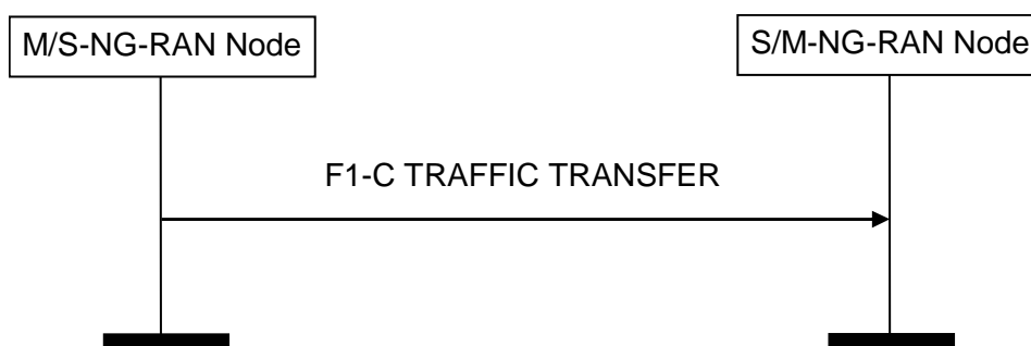
Figure 8.5.1.2-1: F1-C Traffic Transfer procedure, successful operation
