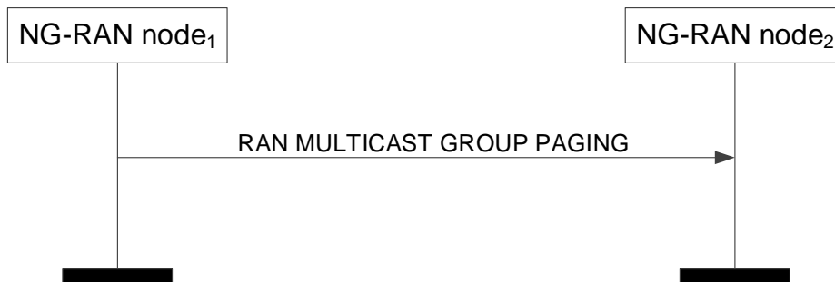
Figure 8.2.11.2-1: RAN Multicast Group Paging, successful operation
