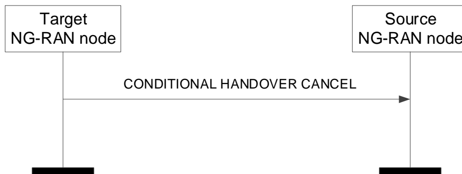
Figure 8.2.9.2-1: Conditional Handover Cancel, successful operation
