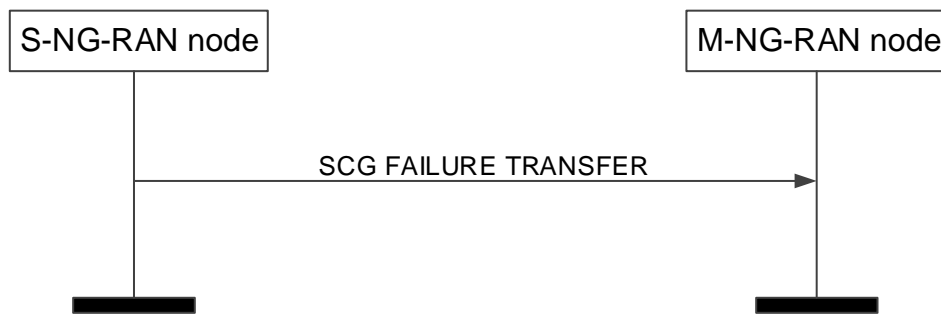
Figure 8.3.18.2-1: SCG Failure Information Transfer, successful operation
