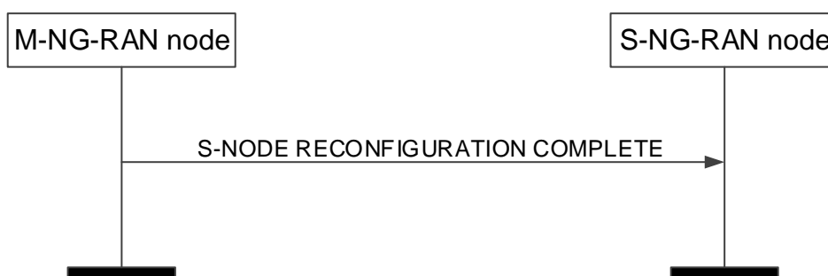
Figure 8.3.2.2-1: S-NG-RAN node Reconfiguration Complete procedure, successful operation.
