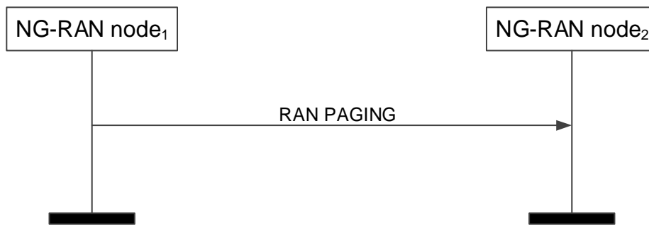
Figure 8.2.5.2-1: RAN Paging: successful operation
