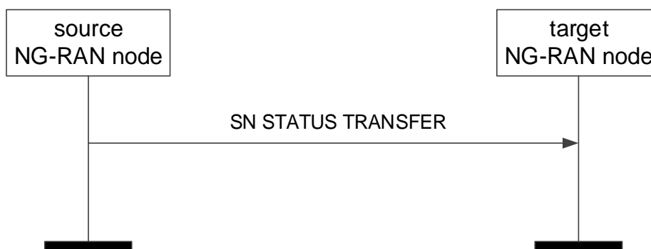
Figure 8.2.2.2-1: SN Status Transfer, successful operation
