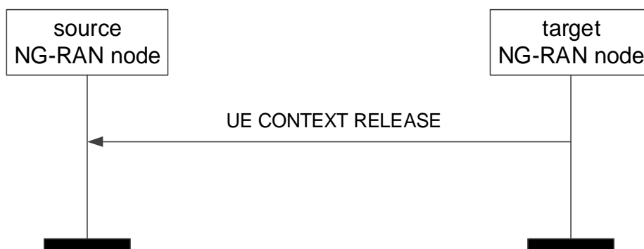
Figure 8.2.7.2-1: UE Context Release, successful operation for handover
