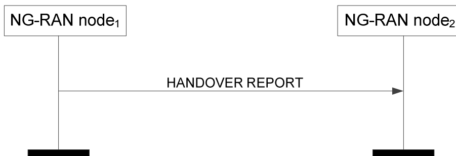
Figure 8.4.8.2-1: Handover Report, successful operation
