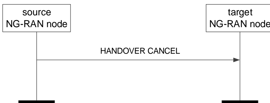
Figure 8.2.3.2-1: Handover Cancel, successful operation
