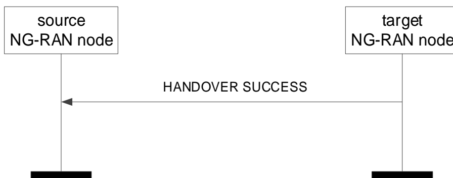
Figure 8.2.8.2-1: Handover Success, successful operation
