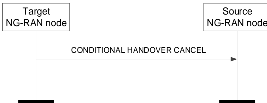
Figure 8.2.9.2-1: Conditional Handover Cancel, successful operation
