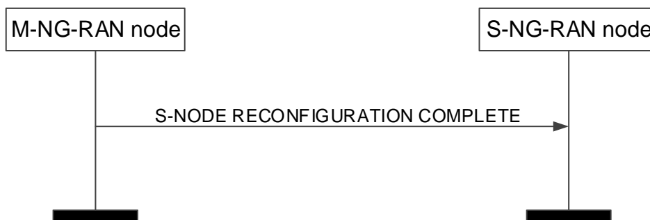
Figure 8.3.2.2-1: S-NG-RAN node Reconfiguration Complete procedure, successful operation.
