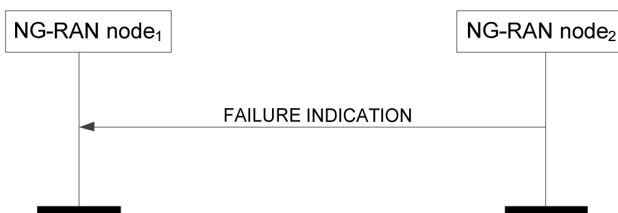
Figure 8.4.7.2-1: Failure Indication, successful operation
