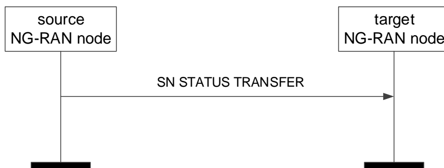
Figure 8.2.2.2-1: SN Status Transfer, successful operation
