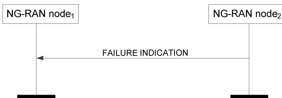
Figure 8.4.7.2-1: Failure Indication, successful operation
