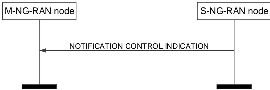
**Figure 8.3.10.3-1: Notification Control Indication procedure, S-NG-RAN node initiated, successful operation.**
