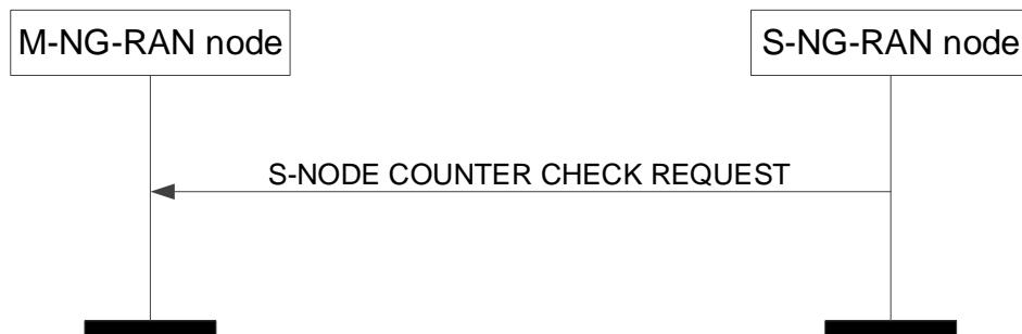
**Figure 8.3.8.2-1: S-NG-RAN node Counter Check procedure, successful operation.**
