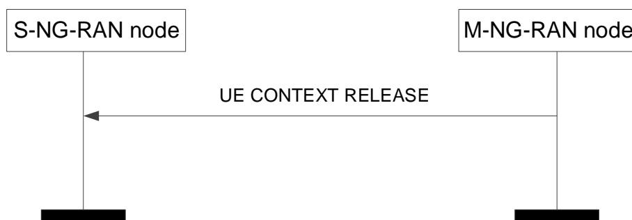
**Figure 8.2.7.2-2: UE Context Release, successful operation for dual connectivity**
