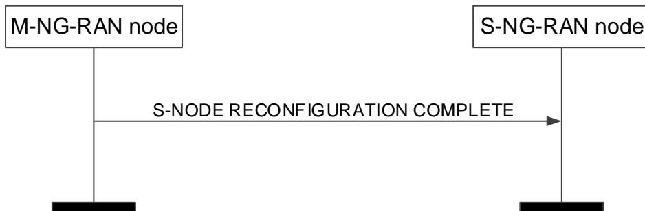
**Figure 8.3.2.2-1: S-NG-RAN node Reconfiguration Complete procedure, successful operation.**
