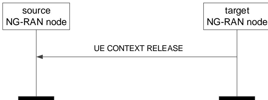
**Figure 8.2.7.2-1: UE Context Release, successful operation for handover**
