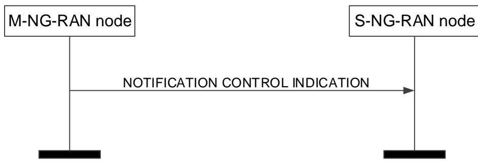
**Figure 8.3.10.2-1: Notification Control Indication procedure, M-NG-RAN node initiated, successful operation.**
