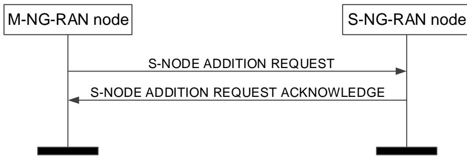
**Figure 8.3.1.2-1: S-NG-RAN node Addition Preparation, successful operation**
