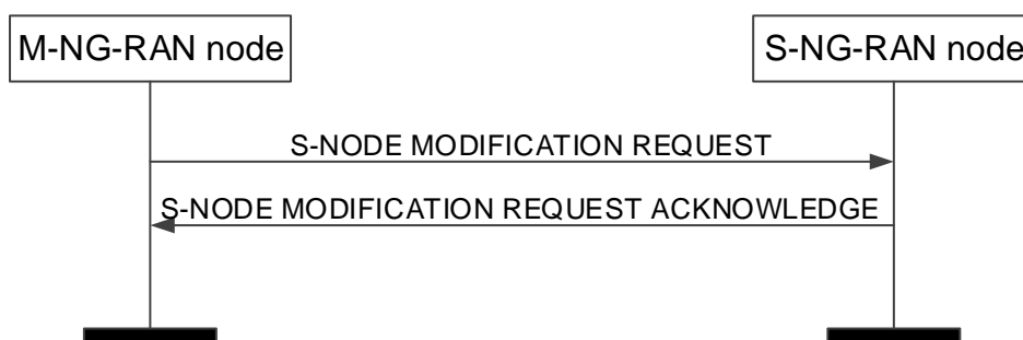
Figure 8.3.3.2-1: M-NG-RAN node initiated S-NG-RAN node Modification Preparation, successful operation
