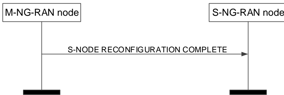
Figure 8.3.2.2-1: S-NG-RAN node Reconfiguration Complete procedure, successful operation.
