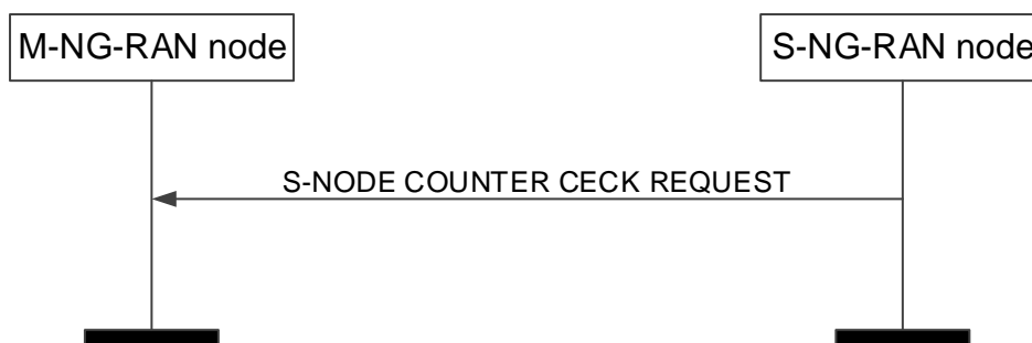
Figure 8.3.8.2-1: S-NG-RAN node Counter Check procedure, successful operation.
