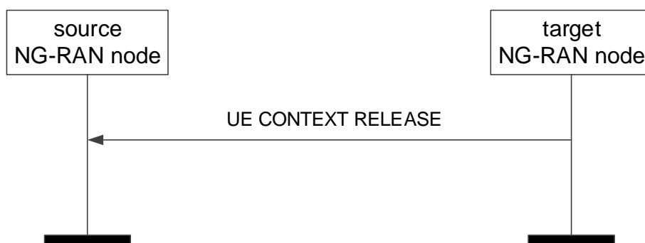
Figure 8.2.7.2-1: UE Context Release, successful operation for handover
