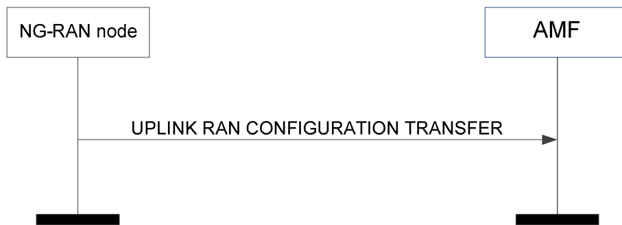
Figure 8.8.1.2-1: Uplink RAN configuration transfer
