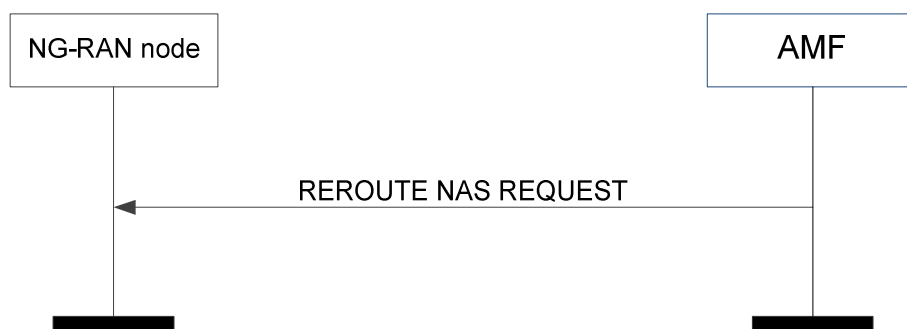
Figure 8.6.5.2-1: Reroute NAS request
