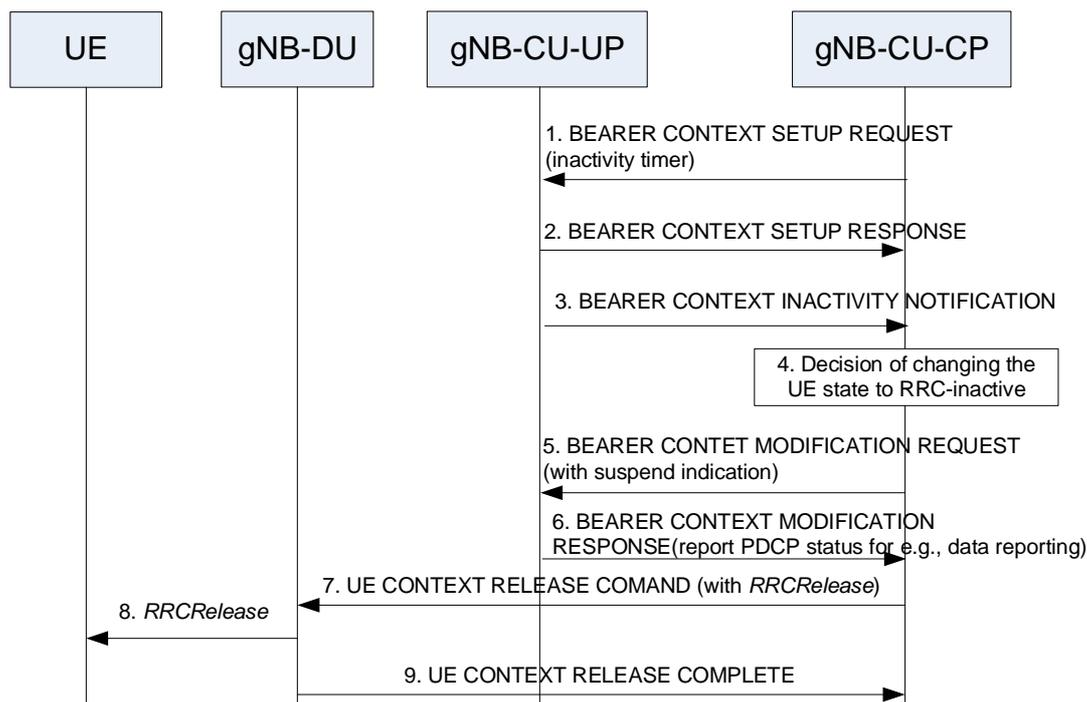
**Figure 8.9.6.1-1: RRC Connected to RRC Inactive state transition.**
