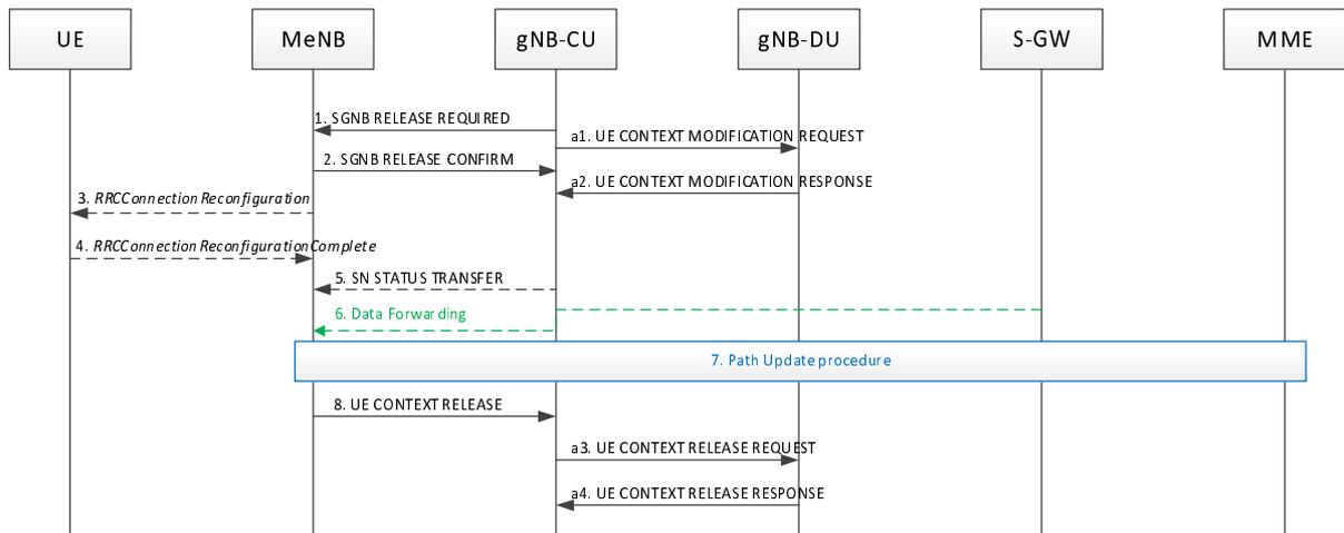
**Figure 8.4.2.1-2 SgNB release procedure in EN-DC (SN initiated)**
