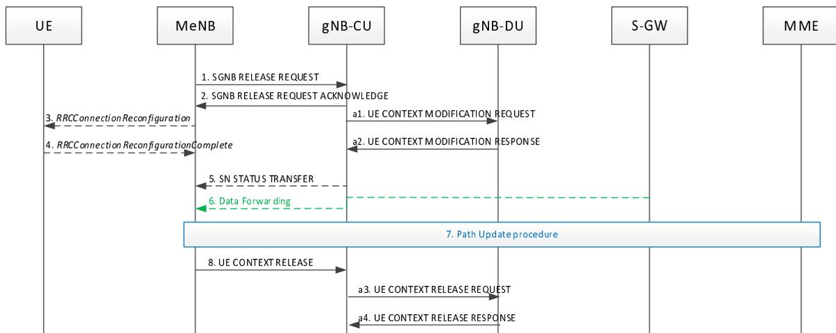
Figure 8.4.2.1-1 SgNB release procedure in EN-DC (MN initiated)
