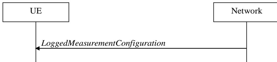
**Figure 5.5a.1.1-1: Logged measurement configuration**
