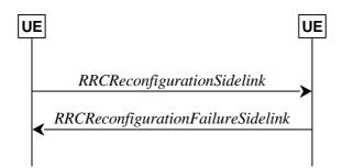
Figure 5.8.9.1.1-2: Sidelink RRC reconfiguration, failure
