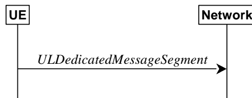
Figure 5.7.7.1-1: UL message segment transfer
