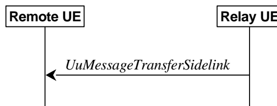
Figure 5.8.9.9.1-1: Uu message transfer in sidelink
