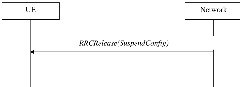
Figure 5.7.15.1-1: SRS For Positioning Configuration in RRC INACTIVE Mode
