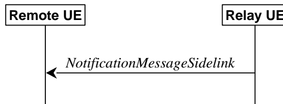
Figure 5.8.9.8.1-1: Notification message in sidelink
