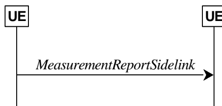
Figure 5.8.10.5.1-1: NR sidelink measurement reporting
