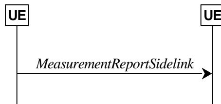
Figure 5.8.10.5.1-1: NR sidelink measurement reporting
