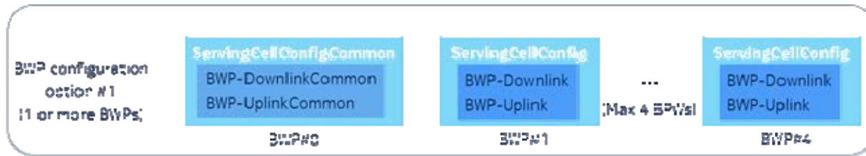
Figure B2-1: BWP#0 configuration without dedicated configuration
