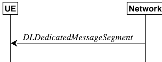
Figure 5.7.6.1-1: DL message segment transfer
