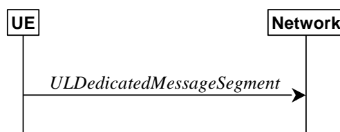
Figure 5.7.7.1-1: UL message segment transfer
