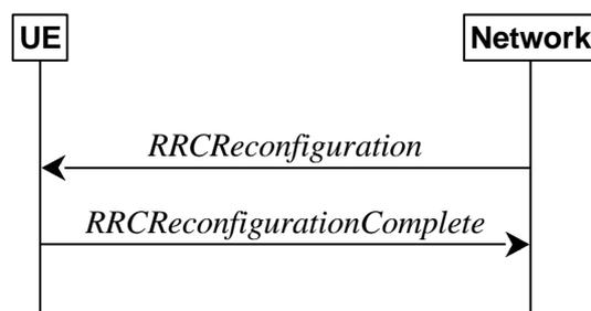
Figure 5.3.5.1-1: RRC reconfiguration, successful
