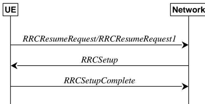
Figure 5.3.13.1-2: RRC connection resume fallback to RRC connection establishment, successful
