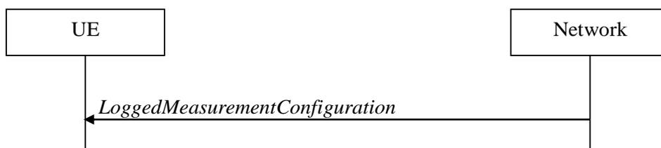
**Figure 5.5a.1.1-1: Logged measurement configuration**
