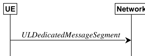
Figure 5.7.7.1-1: UL message segment transfer
