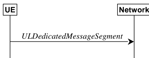
Figure 5.7.7.1-1: UL message segment transfer
