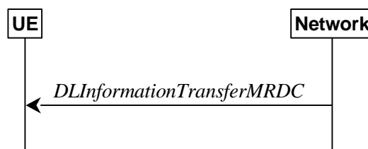
Figure 5.7.1a.1-1: DL information transfer MR-DC
