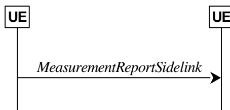
Figure 5.8.10.5.1-1: NR sidelink measurement reporting
