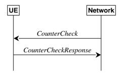
Figure 5.3.6.1-1: Counter check procedure
