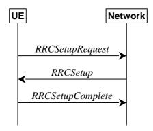
Figure 5.3.3.1-1: RRC connection establishment, successful
