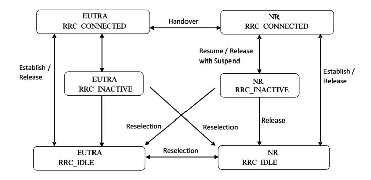
Figure 4.2.1-2: UE state machine and state transitions between NR/5GC, E-UTRA/EPC and E-UTRA/5GC
