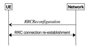
Figure 5.3.5.1-2: RRC reconfiguration, failure
