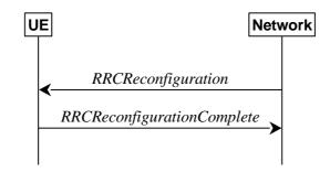
Figure 5.3.5.1-1: RRC reconfiguration, successful
