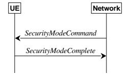
Figure 5.3.4.1-1: Security mode command, successful
