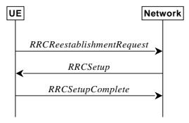
Figure 5.3.7.1-2: RRC re-establishment, fallback to RRC establishment, successful
