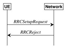
Figure 5.3.3.1-2: RRC connection establishment, network reject
