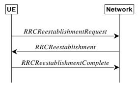
Figure 5.3.7.1-1: RRC connection re-establishment, successful
