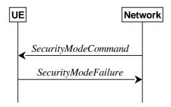
Figure 5.3.4.1-2: Security mode command, failure
