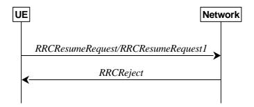
Figure 5.3.13.1-5: RRC connection resume, network reject
