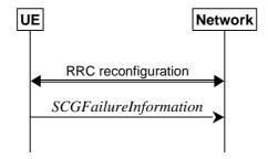
Figure 5.7.3.1-1: SCG failure information
