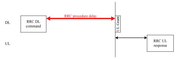
Figure 12.1-1: Illustration of RRC procedure delay
