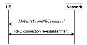
Figure 5.4.3.1-2: Mobility from NR, failure
