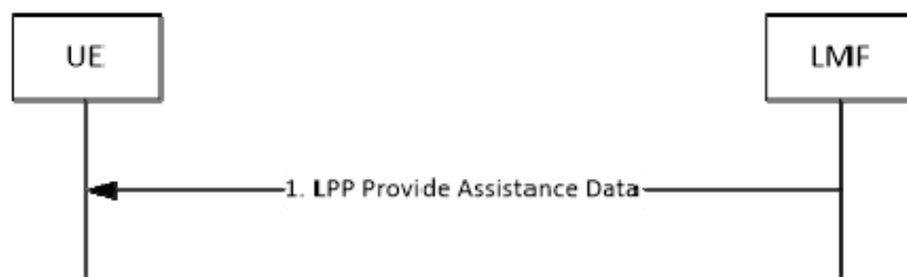
Figure 8.10.3.1.2.1.1-1: LMF-initiated Assistance Data Delivery Procedure
