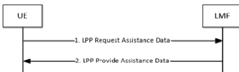
Figure 8.11.3.1.2.2-1: UE-initiated Assistance Data Transfer Procedure
