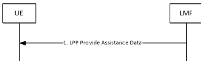
Figure 8.11.3.1.2.1-1: LMF-initiated Assistance Data Delivery Procedure
