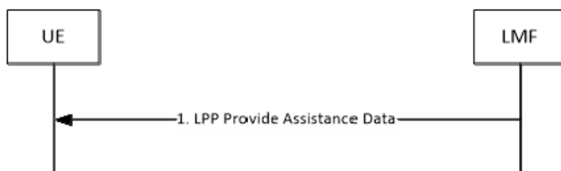
Figure 8.11.3.1.2.1-1: LMF-initiated Assistance Data Delivery Procedure
