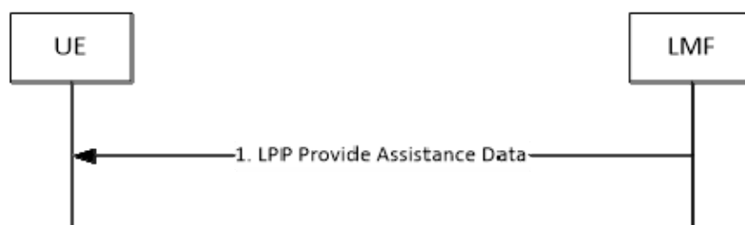
Figure 8.12.3.1.2.1-1: LMF-initiated Assistance Data Delivery Procedure
