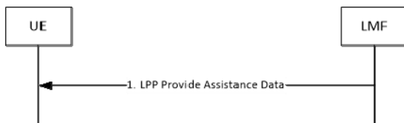
Figure 8.10.3.1.2.1.1-1: LMF-initiated Assistance Data Delivery Procedure
