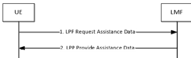
Figure 8.6.3.2.2-1: UE-initiated Assistance Data Transfer Procedure
