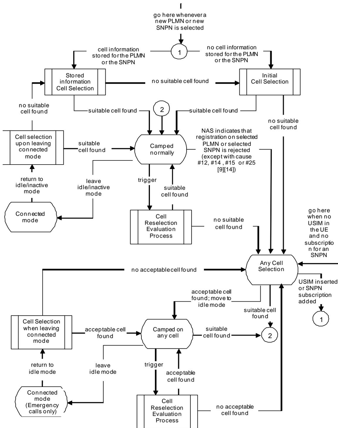
Figure 5.2.2-1: RRC\_IDLE and RRC\_INACTIVE Cell Selection and Reselection
