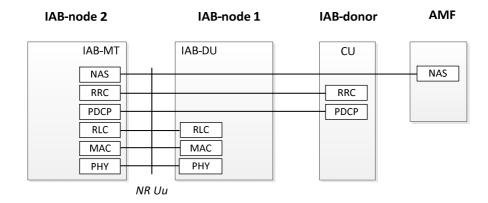
Figure 4.7.2-3: Protocol stack for the support of IAB-MT's RRC and NAS connections
