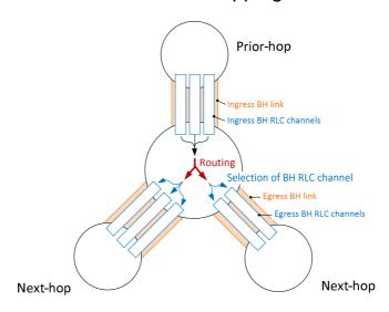
Figure 6.11.3-1: Routing and BH RLC channel selection on BAP sublayer
