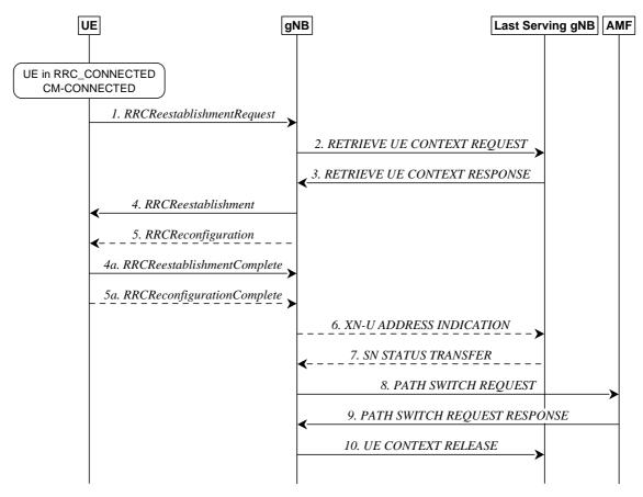
Figure 9.2.3.3-1: Re-establishment procedure
