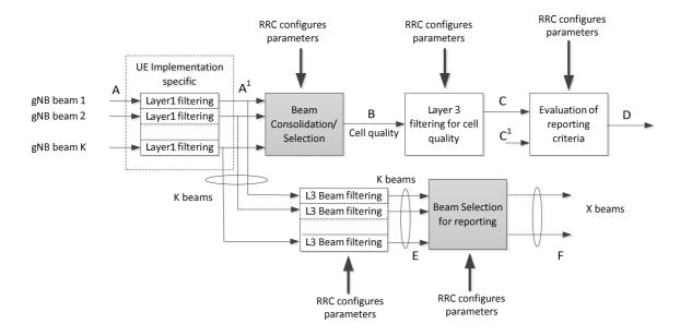
Figure 9.2.4-1: Measurement Model
