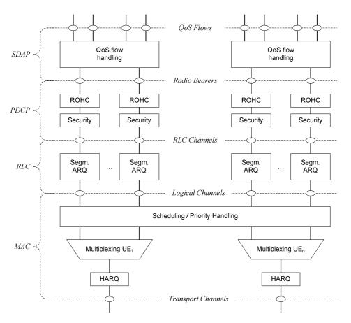
Figure 6.1-1: Downlink Layer 2 Structure
