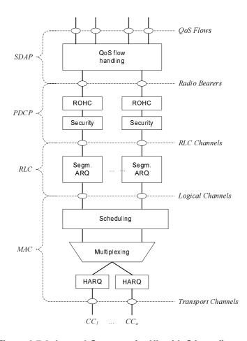
Figure 6.7-2: Layer 2 Structure for UL with CA configured
