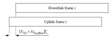
Figure 5.1-2: Uplink-downlink timing relation
