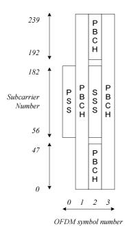
Figure 5.2.4-1: Time-frequency structure of SSB
