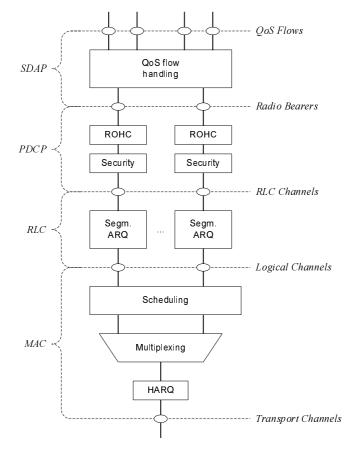
Figure 6.1-2: Uplink Layer 2 Structure
