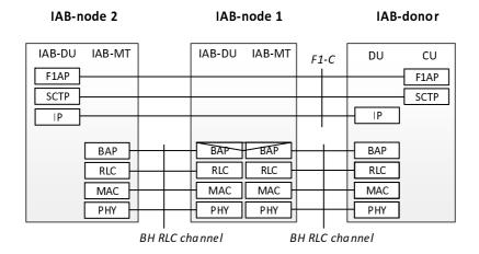
Fig. 4.7.2-2: Protocol stack for the support of F1-C protocol
