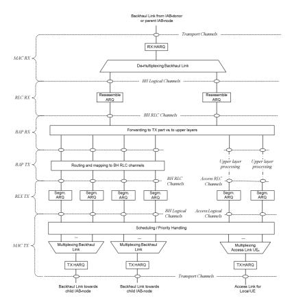
Figure 6.1-4: DL L2-structure at IAB-node
