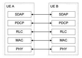
Figure 16.9.2.1-4: User plane protocol stack for STCH.
