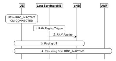
Figure 9.2.2.4.2-1: Network triggered transition from RRC\_INACTIVE to RRC\_CONNECTED
