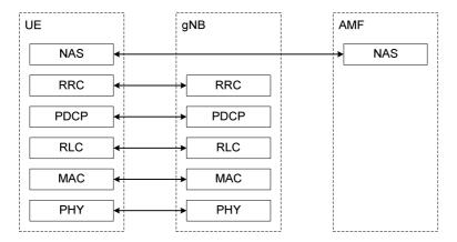
Figure 4.4.2-1: Control Plane Protocol Stack
