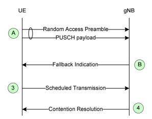
Figure 9.2.6-2: Fallback for CBRA with 2-step RA type
