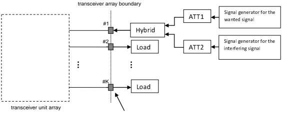
Transceiver array boundary connector TAB(n)
