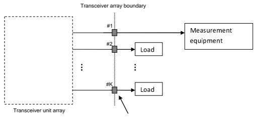
Transceiver array boundary connector TAB(n)
