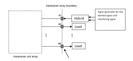
Figure D.2.5-1: Measuring system set-up for IAB type 1-H in-channel selectivity test
