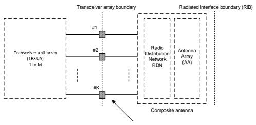
Transceiver array boundary connector (TAB)
