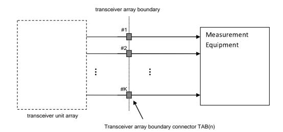
Figure D.1.1-2: Measuring system set-up for *IAB type 1-H* output power, output power dynamics, transmitter ON/OFF power, frequency error, EVM, unwanted emissions for multiple *TAB connectors*
