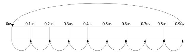
Figure 8.1.4.1.4.2-2: Timing offset scheme for PRACH preamble format 0
