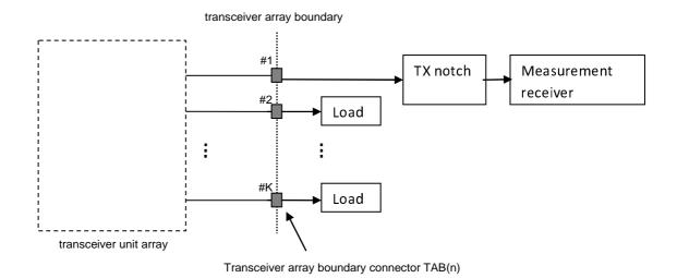
Figure D.2.4-1: Measuring system set-up for *IAB type 1-H* receiver spurious emissions for a single *TAB connector*
