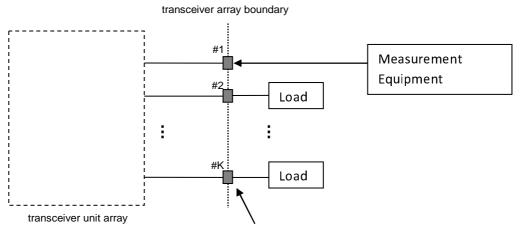
Transceiver array boundary connector TAB(n)
