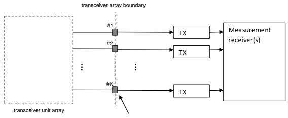
Transceiver array boundary connector TAB(n)
