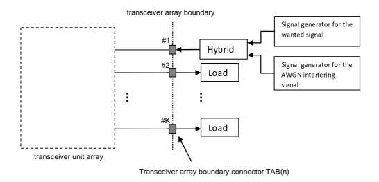
Figure D.2.2-1: Measuring system set-up for IAB type 1-H dynamic range test
