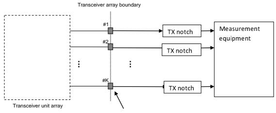
Transceiver array boundary connector TAB(n)
