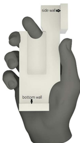
Figure 6.2.2-1: Right-handed PDA Grip hand phantom with a spacer
