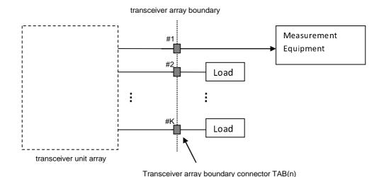
Figure 4.5.2.1-1: Transmitter test ports
