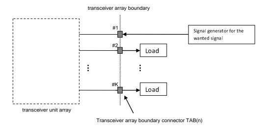
Figure D.4.1-1: Measuring system set-up for BS type 1-H reference sensitivity level test
