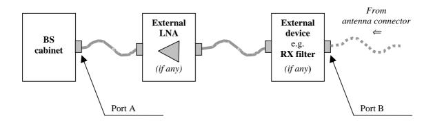
Figure 4.2.1-2: BS type 1-C receiver interface
