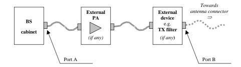
Figure 4.2.1-1: BS type 1-C transmitter interface
