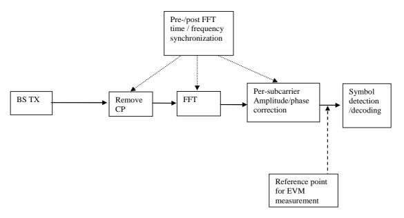
Figure H.2.4-1: Reference point for FR1 EVM measurements
