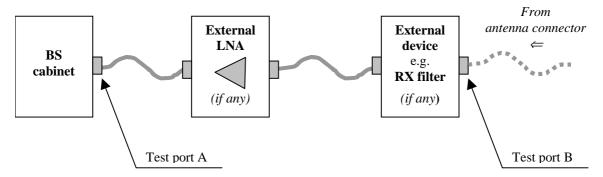
Figure 4.5.1.2.1-1: Receiver test ports
