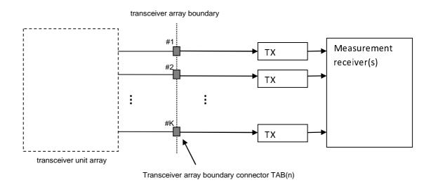
Figure D.4.4-2: Measuring system set-up for *BS type 1-H* receiver spurious emissions for multiple *TAB connectors*
