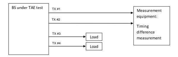
Figure D.1.3-1: Measuring system set-up for BS type 1-C test of time alignment error
