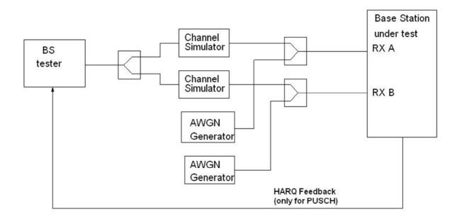
Figure D.5.1-1: Functional set-up for performance requirements for PUSCH, single user PUCCH, PRACH on single antenna port in multipath fading conditions and for High Speed Train conditions for BS with Rx diversity (2 Rx case shown)
