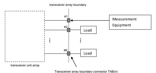
Figure 4.5.2.2-1: Receiver test ports
