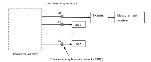
Figure D.4.4-1: Measuring system set-up for *BS type 1-H* receiver spurious emissions for a single *TAB connector*
