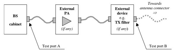
Figure 4.5.1.1.1-1: Transmitter test ports
