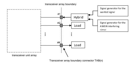
Figure D.4.2-1: Measuring system set-up for BS type 1-H dynamic range test
