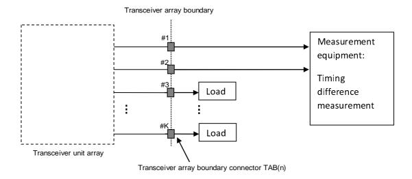
Figure D.3.4-1: Measuring system set-up for BS type 1-H test of time alignment error
