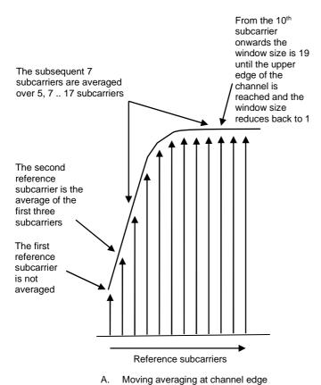
Figure B shows an example of 1RB allocation using a reduced window size of five subcarriers for averaging. The same method applies for RB allocations with fewer than 19 subcarriers available for the moving average size. For the case of 2 and 3 RB allocations, 11 and 17 are the window sizes, respectively.
