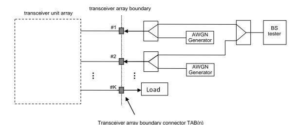
Figure D.6.3-1: Functional set-up for performance requirements for PUSCH and PRACH in static conditions for BS with Rx diversity (2 Rx case shown)
