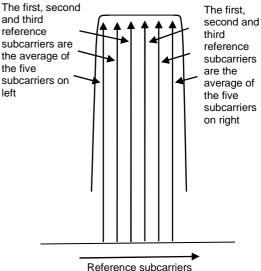
B. Moving averaging for the case when the number of available reference subcarriers within a set of contiguously allocated RBs is smaller than the moving average window size
