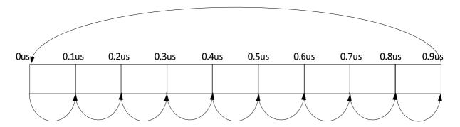
Figure 8.4.1.4.2-2: Timing offset scheme for PRACH preamble format 0
