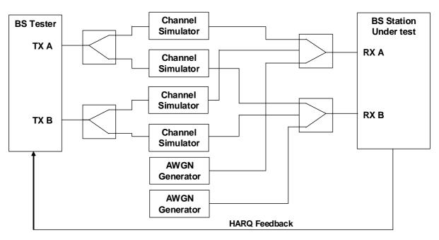
Figure D.5.2-1: Functional set-up for performance requirements for PUSCH transmission on two antenna ports in multipath fading conditions (2 Rx case shown)
