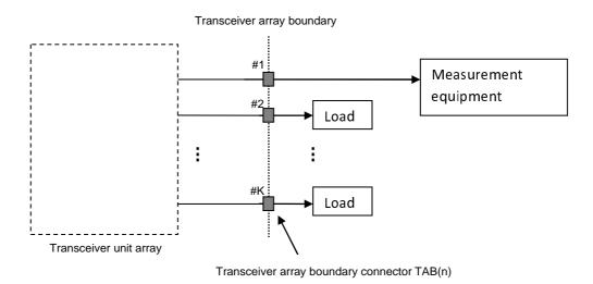
Figure D.3.1-1: Measuring system set-up for *BS type 1-H* output power, output power dynamics, transmitter ON/OFF power, frequency error, EVM, unwanted emissions for a single *TAB connector*
