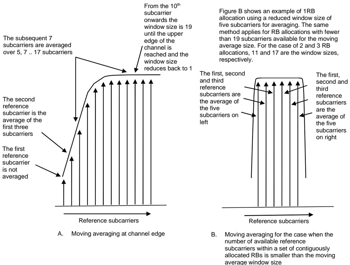
Figure B.6-1: Reference subcarrier smoothing in the frequency domain
