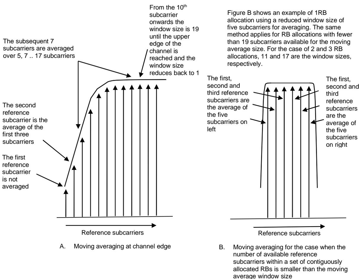
Figure C.6-1: Reference subcarrier smoothing in the frequency domain
