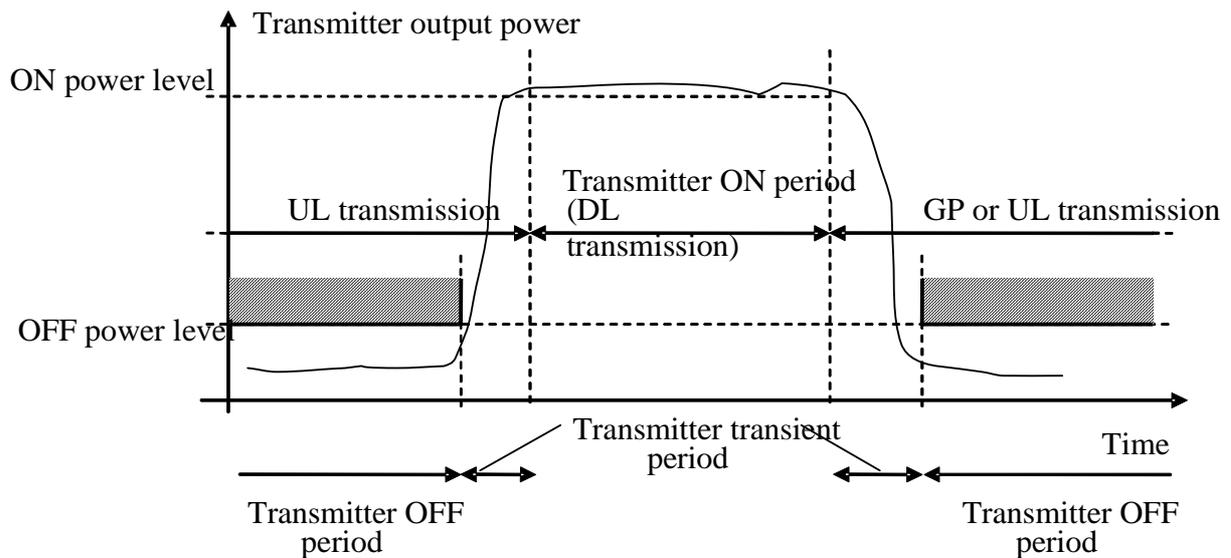
**Figure 6.4.2.1-1: Example of relations between *transmitter ON period*, *transmitter OFF period* and *transmitter transient period***
