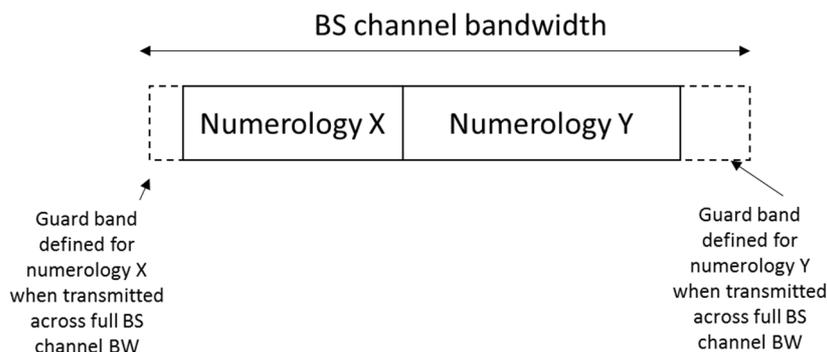
**Figure 5.3.3-2: Guard band definition when transmitting multiple numerologies**
