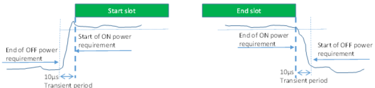
Figure 9.3.3.2-1a: General ON/OFF time mask for NR UL transmission in FR1-NTN above 10 GHz
