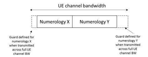
Figure 5.3.3-3: Guard band definition when transmitting multiple numerologies
