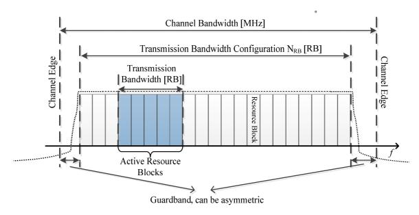
Figure 5.3.1-1: Definition of the channel bandwidth and the maximum transmission bandwidth configuration for one channel
