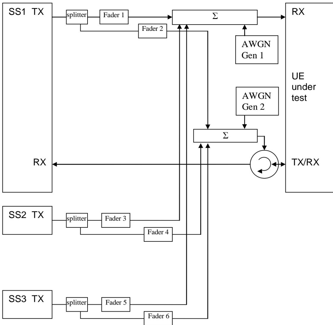
Figure A.4: Connection for 3 cells OTDOA tests with multipath fading propagation conditions
