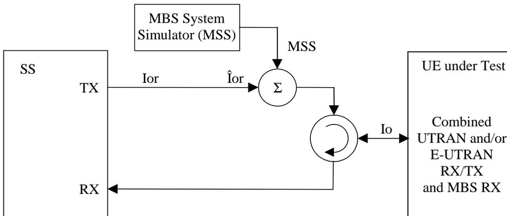
**Figure A.6: Connection for MBS Minimum Performance requirements tests for UE with combined UTRAN and/or E-UTRAN / MBS antenna**
