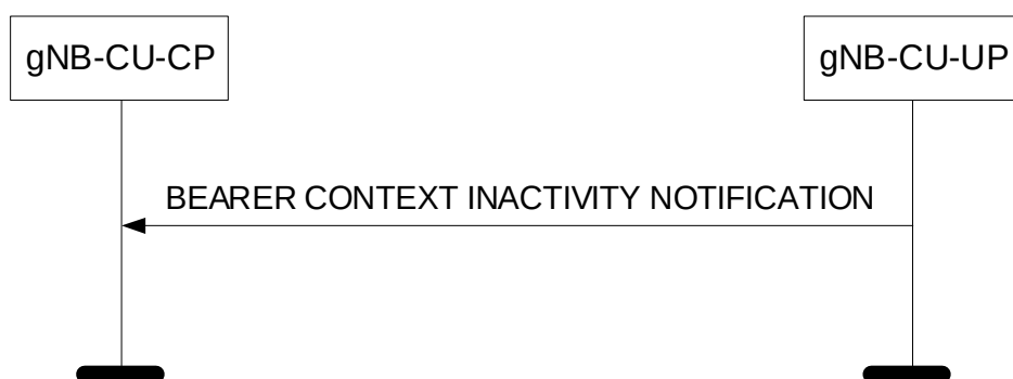
Figure 8.3.6.2-1: Bearer Context Inactivity Notification procedure: Successful Operation.
