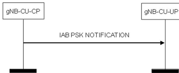
Figure 8.5.2.2-1: IAB PSK Notification procedure: Successful Operation.
