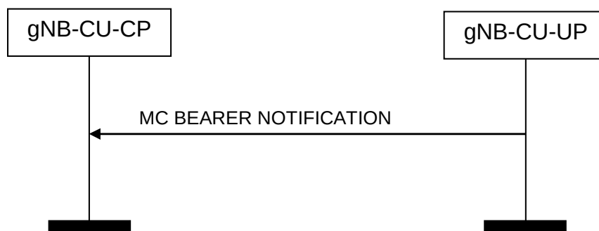
Figure 8.6.2.6.2-1: MC Bearer Notification procedure: Successful Operation.
