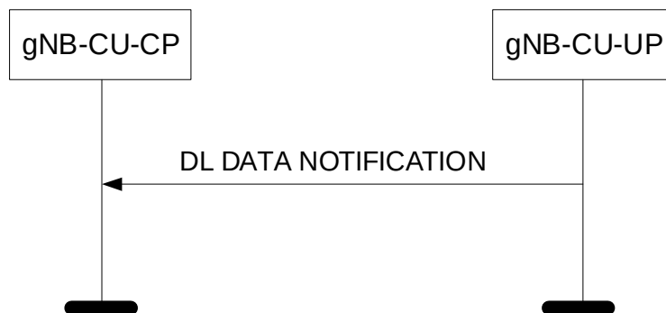
Figure 8.3.7.2-1: DL Data Notification procedure: Successful Operation.
