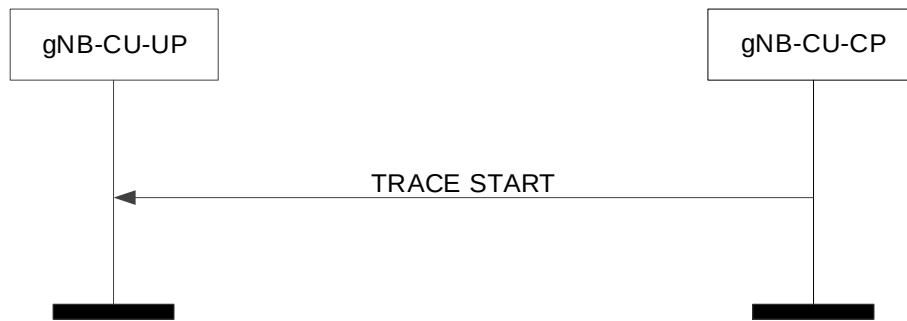
Figure 8.4.1.2-1: Trace start procedure: Successful Operation.
