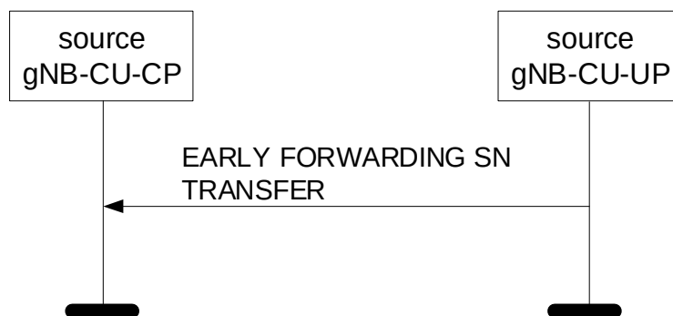
Figure 8.3.12.2-1: Early Forwarding SN Transfer procedure: Successful Operation.
