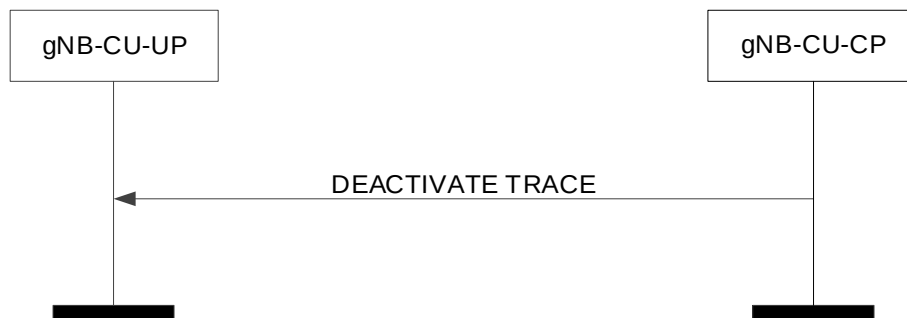
Figure 8.4.2.2-1: Deactivate trace procedure: Successful Operation.
