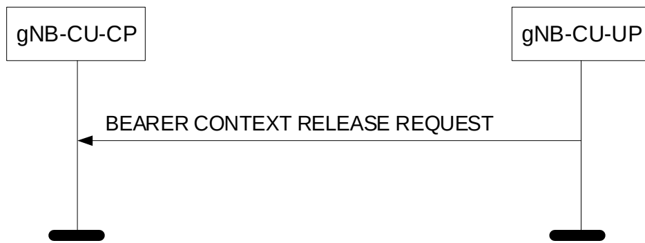
Figure 8.3.5.2-1: Bearer Context Release Request procedure: Successful Operation.
