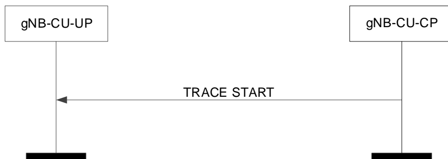
Figure 8.4.1.2-1: Trace start procedure: Successful Operation.
