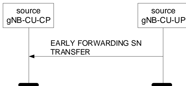
Figure 8.3.12.2-1: Early Forwarding SN Transfer procedure: Successful Operation.
