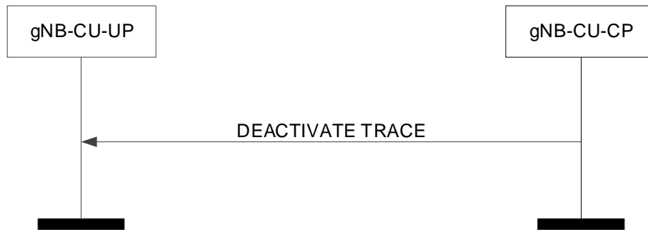
Figure 8.4.2.2-1: Deactivate trace procedure: Successful Operation.
