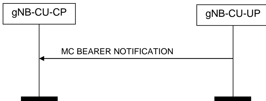
Figure 8.6.2.6.2-1: MC Bearer Notification procedure: Successful Operation.
