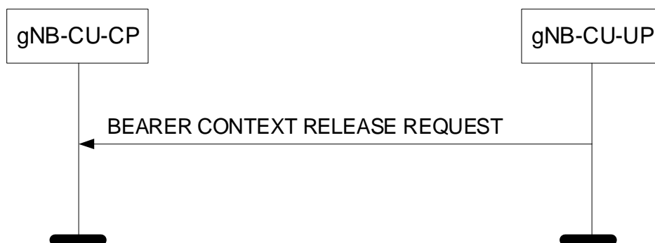
Figure 8.3.5.2-1: Bearer Context Release Request procedure: Successful Operation.
