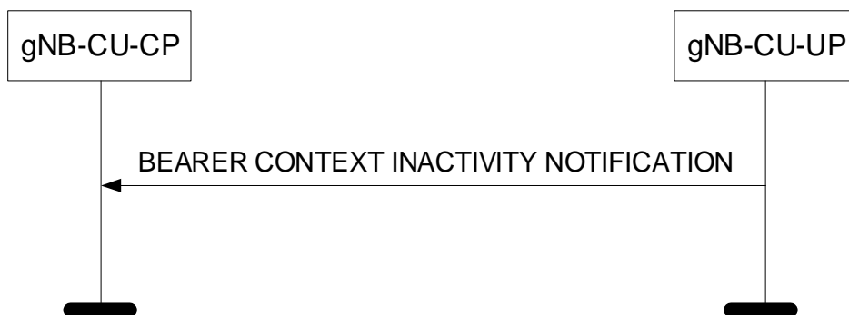
Figure 8.3.6.2-1: Bearer Context Inactivity Notification procedure: Successful Operation.
