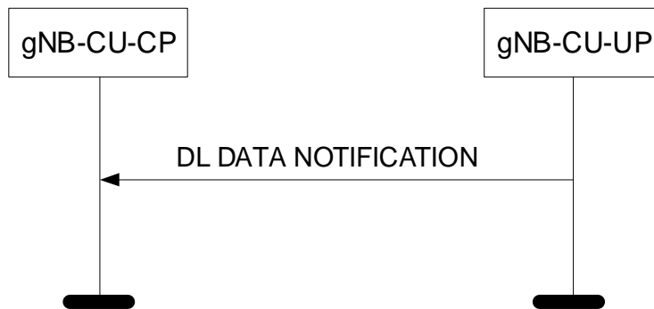
Figure 8.3.7.2-1: DL Data Notification procedure: Successful Operation.
