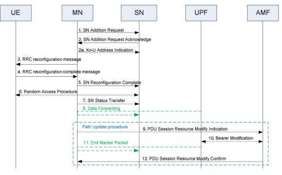
Figure 10.2.2-1: SN Addition procedure
