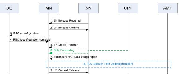
Figure 10.4.2-2: SN release procedure - SN initiated
