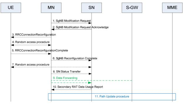
Figure 10.3.1-1: SN Modification procedure - MN initiated
