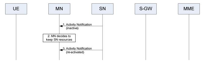
Figure 10.12.1-1: Support of Activity Notification in EN-DC
