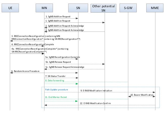
Figure 10.2.1-2: Conditional Secondary Node Addition procedure
