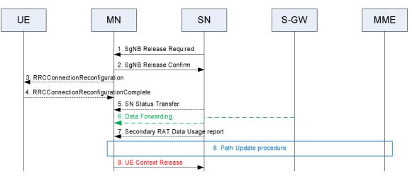
Figure 10.4.1-2: SN Release procedure – SN initiated
