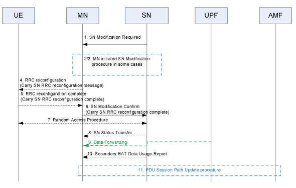
Figure 10.3.2-2: SN Modification procedure - SN initiated with MN involvement
