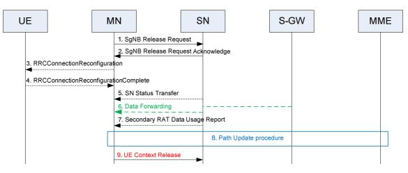
Figure 10.4.1-1: SN Release procedure – MN initiated
