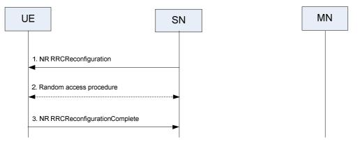
Figure 10.3.1-3: SN modification - SN initiated without MN involvement
