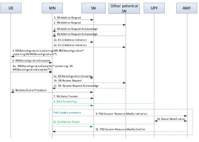
Figure 10.2.2-2: Conditional Secondary Node Addition procedure
