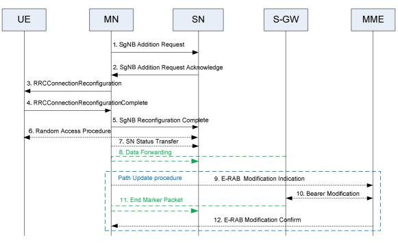
Figure 10.2.1-1: Secondary Node Addition procedure
