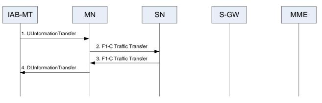
Figure 10.15-1: F1-C transfer procedure in EN-DC
