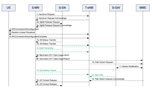
Figure 10.8.1-1: Master Node to eNB Change procedure
