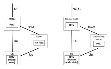
Figure 4.2.1-1: Control plane architecture for EN-DC (left) and MR-DC with 5GC (right).
