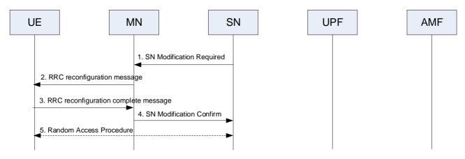
Figure 10.3.2-4: Transfer of an NR RRC message to/from the UE
