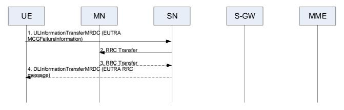
Figure 10.10.1-4: RRC Transfer procedure for MCG failure information
