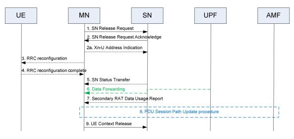
Figure 10.4.2-1: SN release procedure - MN initiated
