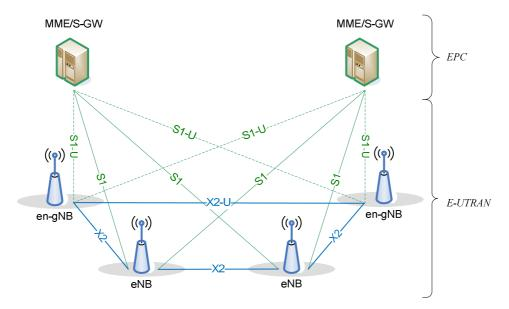
Figure 4.1.2-1: EN-DC Overall Architecture
