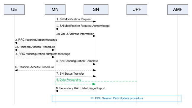
Figure 10.3.2-1: SN Modification procedure - MN initiated
