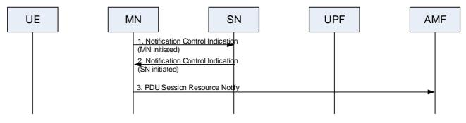
Figure 10.13.2-1: Notification Control Indication procedure
