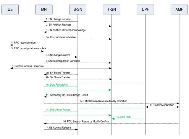
Figure 10.5.2-2: SN change procedure - SN initiated
