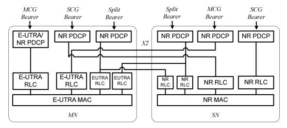
Figure 4.2.2-3: Network side protocol termination options for MCG, SCG and split bearers in MR-DC with EPC (EN-DC).
