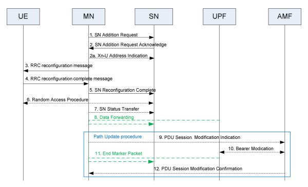
Figure 10.2.2-1: SN Addition procedure
