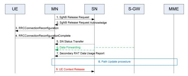
Figure 10.4.1-1: SN Release procedure - MN initiated
