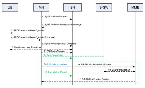
Figure 10.2.1-1: Secondary Node Addition procedure
