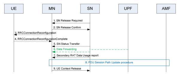
Figure 10.4.2-2: SN release procedure - SN initiated
