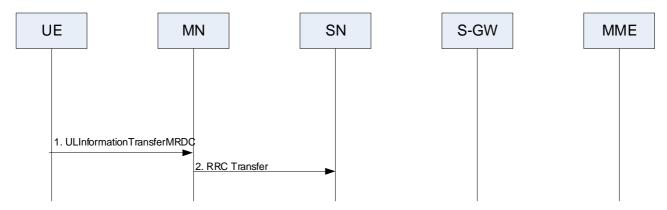
Figure 10.10.1-3: RRC Transfer procedure for NR measurement report or NR failure information
