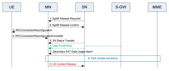
Figure 10.4.1-2: SN Release procedure - SN initiated
