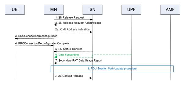
Figure 10.4.2-1: SN release procedure - MN initiated
