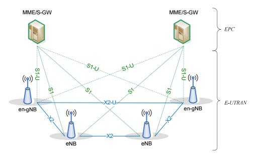
Figure 4.1.2-1: EN-DC Overall Architecture
