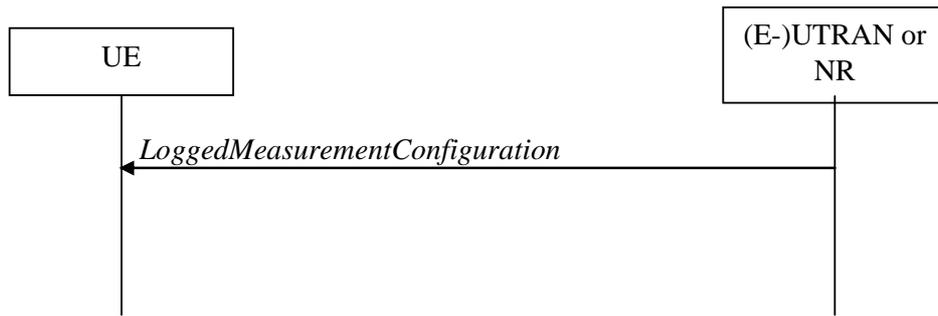
**Figure 5.1.1.1-1: MDT measurement configuration for Logged MDT**
