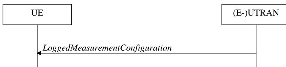
**Figure 5.1.1.1-1: MDT measurement configuration for Logged MDT**
