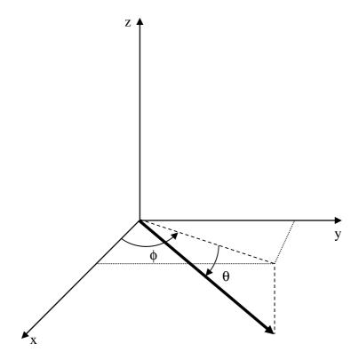
Figure 4.14-1: Reference coordinate system
