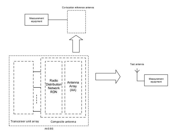
Figure 4.8.1-2: Transmitter test interfaces for co-location concept
