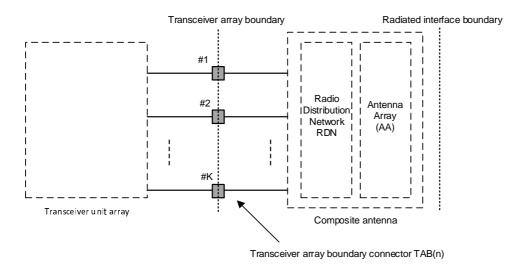
Figure 4.2-1: Radiated and conducted points of reference of hybrid AAS BS
