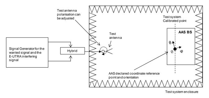
Figure D.2.7-1: Measurement set up for OTA In-channel selectivity
