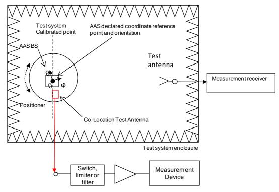
Figure D.1.4-1: Measurement set up for OTA Co-location emissions, TX OFF power
