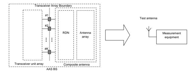
Figure 4.8.1-1: Transmitter test interfaces
