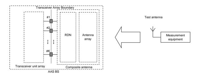
Figure 4.8.2-1: Receiver test interfaces
