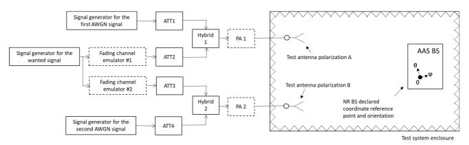
Figure D.3-2: Measurement set up for single TX, dual polarization radiated performance requirements
