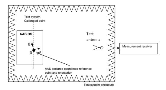
Figure D.1.1-1: Measurement set up for Radiated Transmit Power, OTA E-UTRA DL RS power, output power dynamics, Transmitter signal quality
