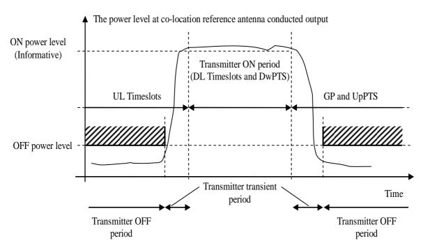
Figure 6.5.3.1-1: Illustration of the relations of transmitter ON period, transmitter OFF period and transmitter transient period
