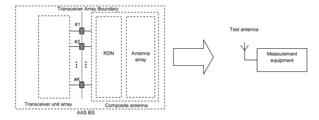
Figure 4.8.1-1: Transmitter test interfaces
