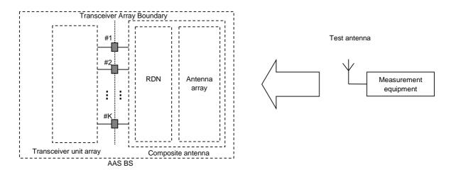
Figure 4.8.2-1: Receiver test interfaces
