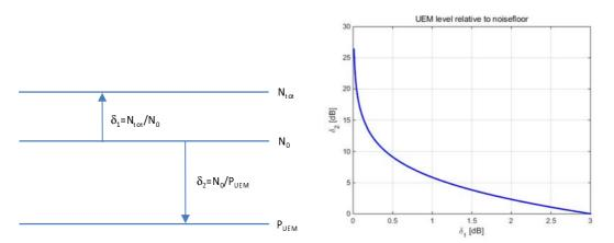
Figure H-1: Relative noise measurement
