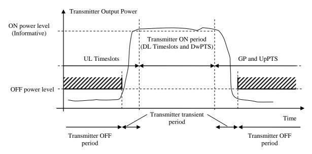
Figure 6.4.3.1-1: Illustration of the relations of transmitter ON period, transmitter OFF period and transmitter transient period
