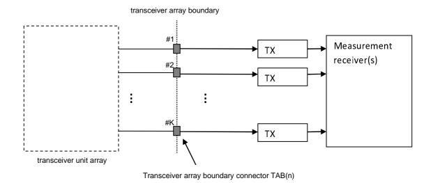
Figure D.2.4-2: Measuring system set-up for receiver spurious emissions for multiple *TAB* connectors
