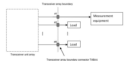
Figure D.1.1-1: Measuring system set-up for AAS BS output power, transmitter ON/OFF power, modulation quality, frequency error and operating band unwanted emissions for a single TAB connector
