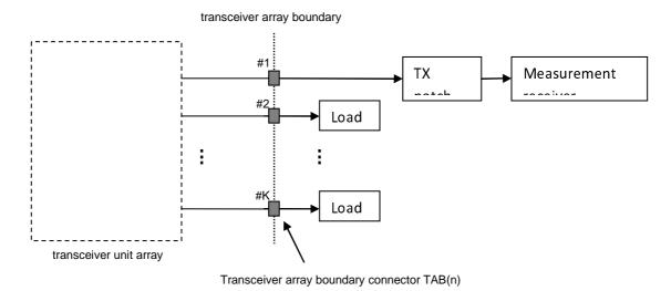
Figure D.2.4-1: Measuring system set-up for receiver spurious emissions for a single TAB connector
