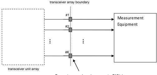
Transceiver array boundary connector TAB(n)
