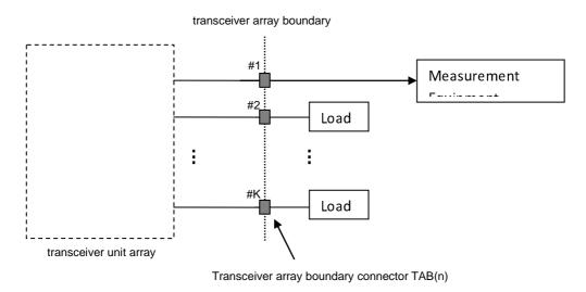
Figure 4.8.1-1: Transmitter test ports
