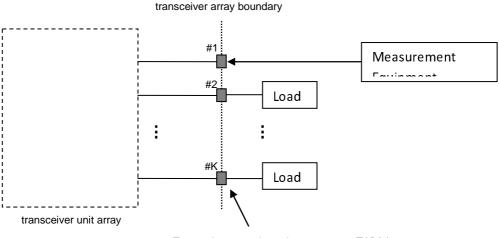
Transceiver array boundary connector TAB(n)
