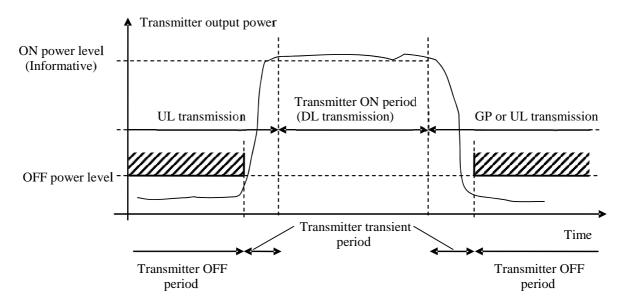
Figure 6.4.1-2: Illustration of the relations of transmitter ON period, transmitter OFF period and transmitter transient period (for NR)
