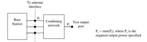
Figure 4.10.7.2-1: Transmitter test set-up
