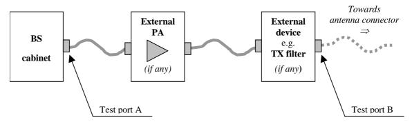
Figure 4.10.1-1: Transmitter test ports
