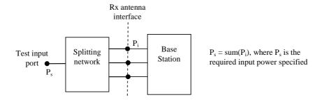
Figure 4.10.7.1-1: Receiver test set-up
