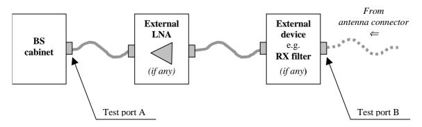
Figure 4.10.2-1: Receiver test ports
