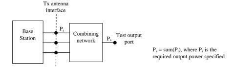
Figure 4.10.7.2-1: Transmitter test set-up
