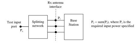
Figure 4.10.7.1-1: Receiver test set-up
