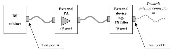
Figure 4.10.1-1: Transmitter test ports
