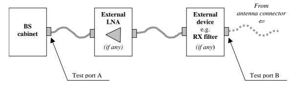
Figure 4.10.2-1: Receiver test ports
