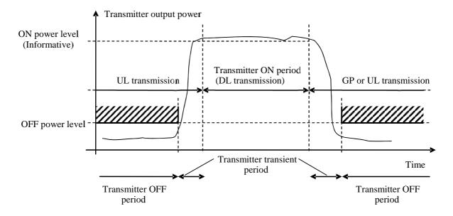
Figure 6.4.1-2: Illustration of the relations of transmitter ON period, transmitter OFF period and transmitter transient period (for NR)
